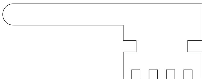
Figure 4.73 Diagram of complex transitional bit
