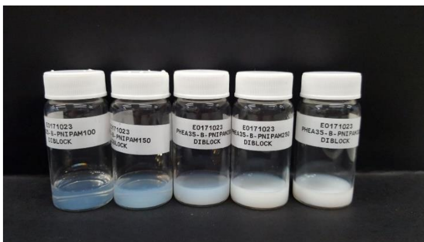
Figure 4.13 – Photograph above the LCST of diblock polymer samples of pHEA_{45}\text{-}b\text{-}pNIPAM_n , with n being 132, 194, 250, 292 and 370 from left to right.
