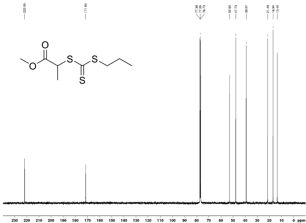
Figure A.4 – 13 C NMR spectrum of MPP RAFT agent recorded in CDCl 3
