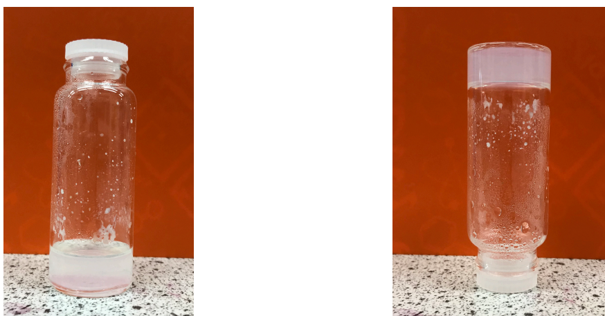
Figure 153: In situ gel during the dimerization of glycolaldehyde phosphate ( 239 ) catalysed by benzylglutamine amide ( 230 )
