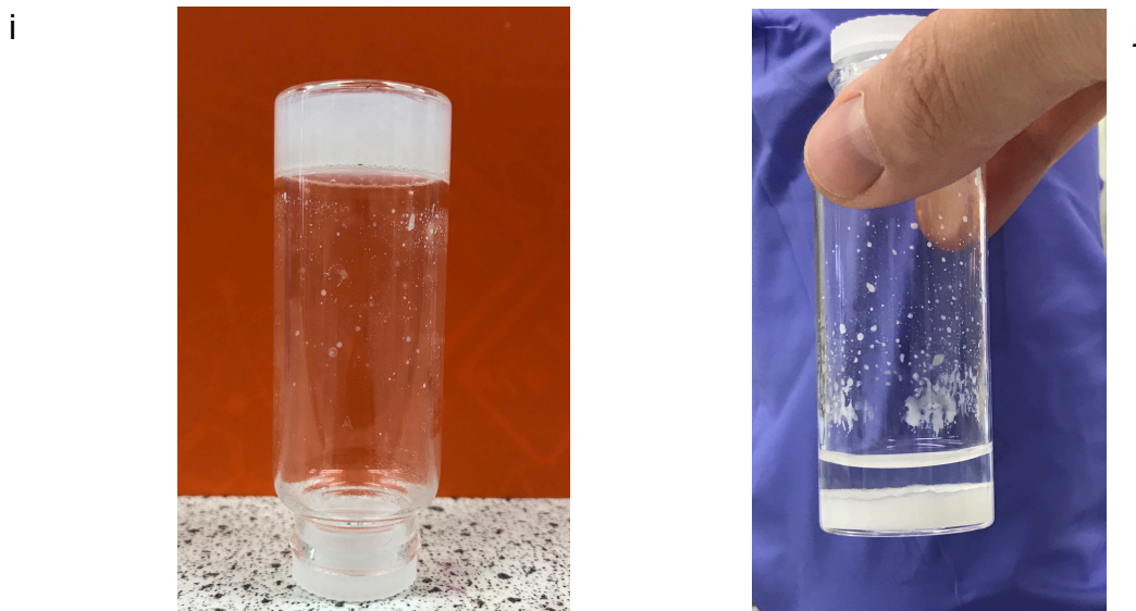
Figure 152: (i) Benzylglutamine amide ( 230 ) gel before reagents loaded, (j) once reagents ( 239 ) added resulting in the loss of the gel network
