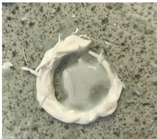
Figure 108: Benzaldehyde and glutamine amide ( 210 ) (5 mg) 1:1 rheology sample prepared using a bottomless vial and sealant.
