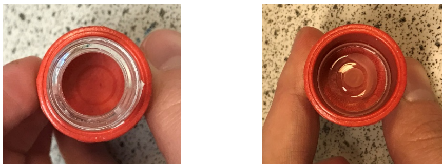
Figure 104: Left bottomless vial in suba-seal, no glass bottom, Right suba-seal with glass bottom
