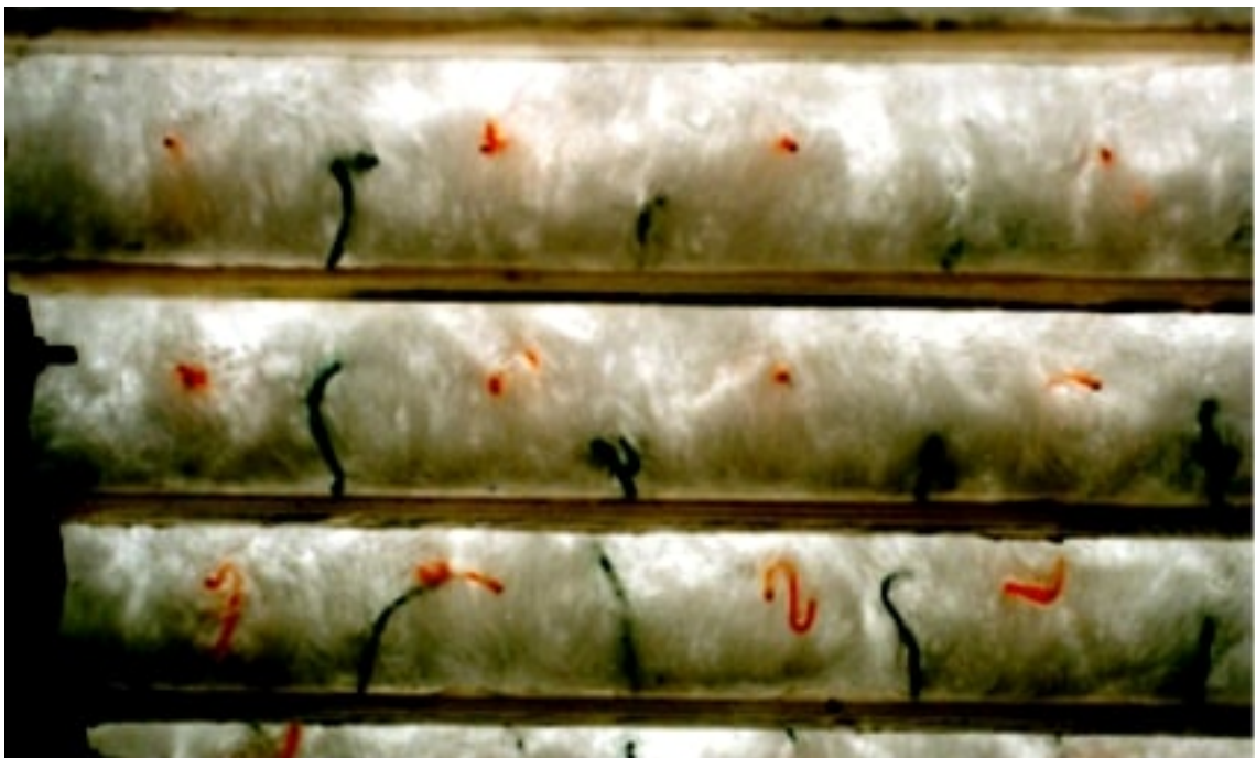
Figure 7.11: Flow with attached wool fibres at the LNEC stepped spillway, viewed from below the chute. Image taken from Matos and Meireles (2014)
