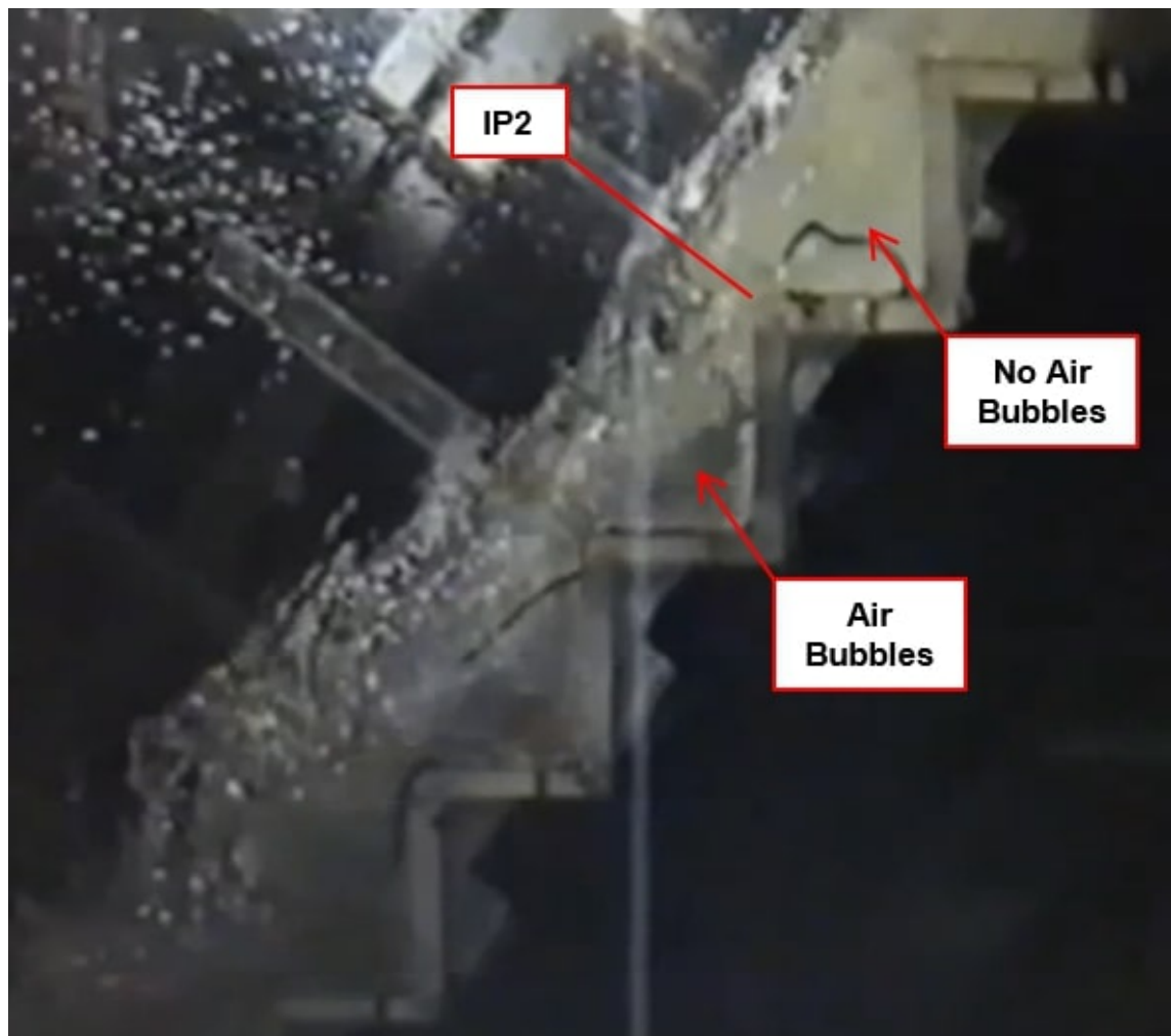
Figure 5.10: View of the visually observed inception point (IP2) from the side of the experimental spillway. The darker regions indicate the presence of air bubbles
