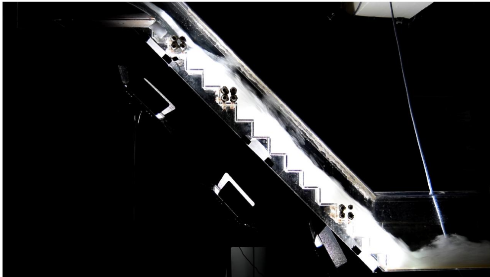
Figure 3.5: One frame of a video used for image analysis to measure the location of the free-surface. Though the use of lighting, background and the ISO of the camera, a sharp contrast between the water and the background is observed at the free-surface
