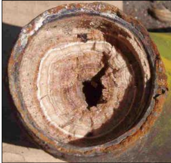
Figure 2.1 Calcium carbonate scale build-up (34)
