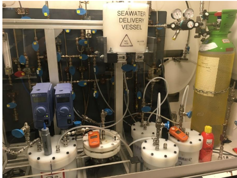
Figure 3.7 Photograph of multiphase scaling rig with H 2 S injection capability and seawater (SW) delivery vessel
