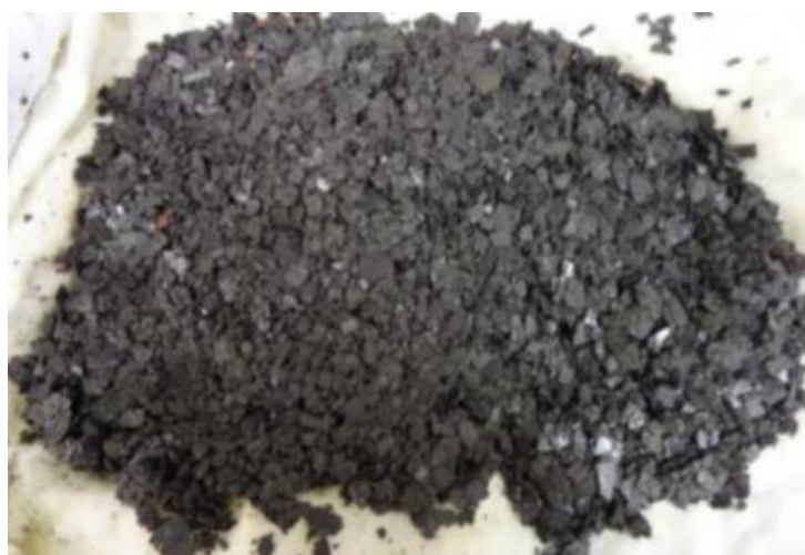
Figure 2.5 Sulphide scale deposits from the North Sea Central Graben fields (38)
