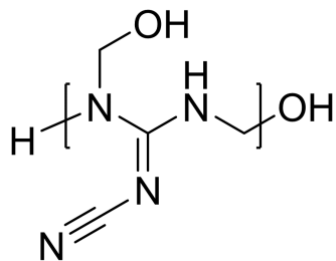
Figure 1-11 Generic structure of dicyandiamide-formaldehyde polymer.
