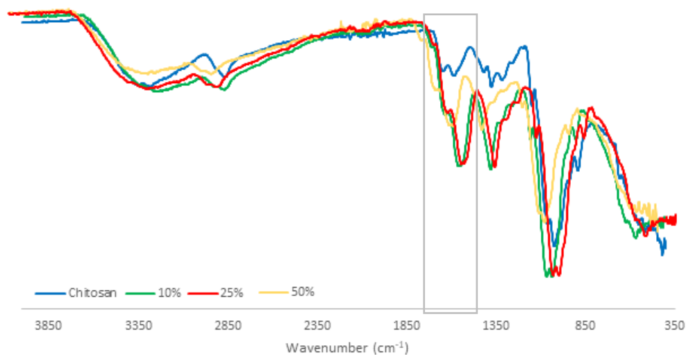
Figure 5-19 A comparison of the FTIR spectra of chitosan to the chitosan modified with citric acid by 10%, 25% and 50%.
