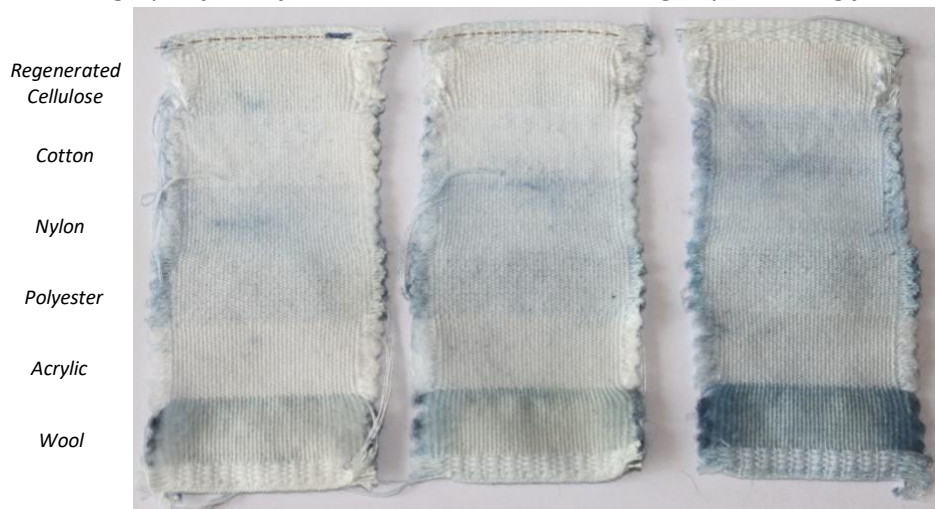
Figure 5-10 Photograph of multifibre swatches washed with indigo dye bleeding fabric. From
