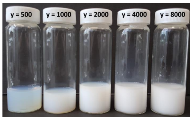
Fig. 5.5. Digital photograph recorded for a series of five 2.5 % w/w aqueous dispersions of PATAc 100 -PDmac y diblock copolymer nanoparticles (where y = 500 – 8000) in 2.0 M ammonium sulfate. Targeting higher PDmac DPs clearly leads to greater turbidity.
