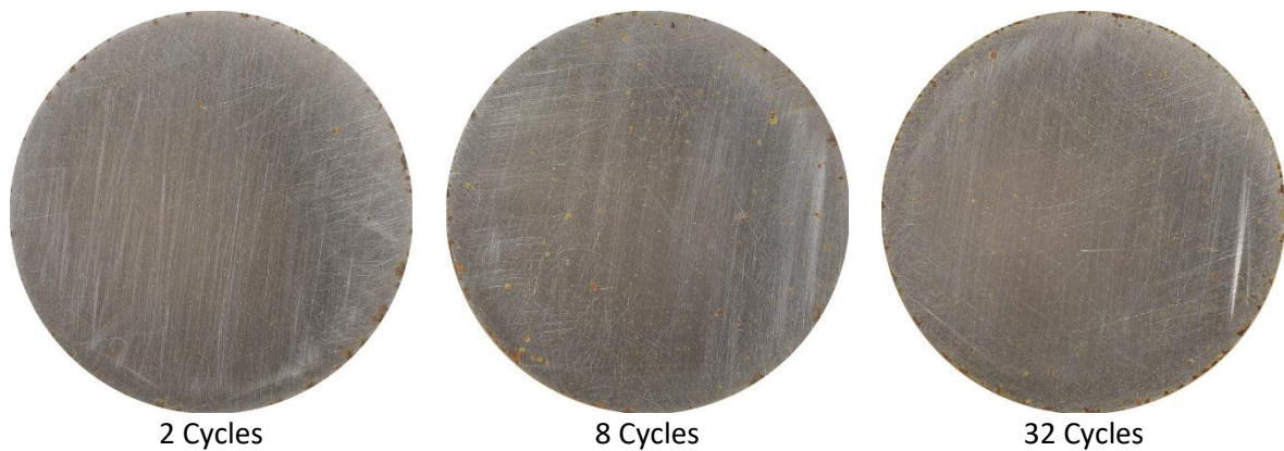
Figure 125, Photographic images taken of samples treated with 2, 8 and 32 cycles of dew / condensation treatment
