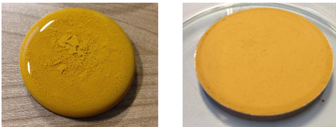
Figure 65, Photographs showing the drying of a goethite oxide dispersion in isopropanol on a sample substrate, left; and the dried sample surface, right
