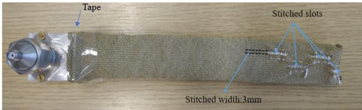
Fig.6.221 Photograph of a knitted SWA with four stitched slots.
