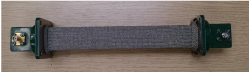
Fig.5.53. Textile sleeve filled with PTFE with WR 90 transitions
