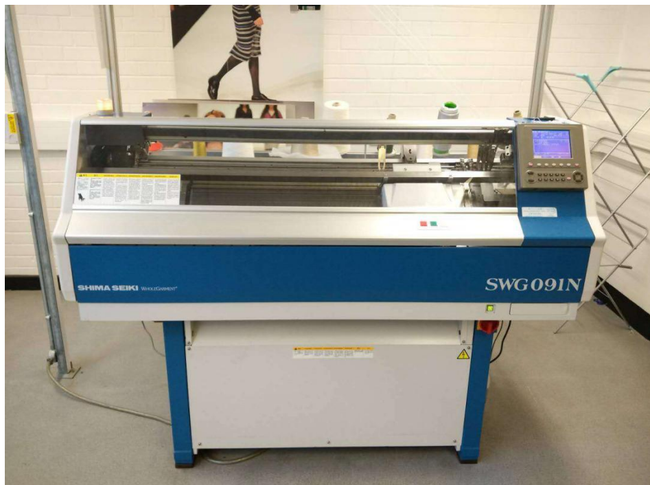
Fig.2.52 A Shima Seiki SWG091N computerized flat-bed knitting
