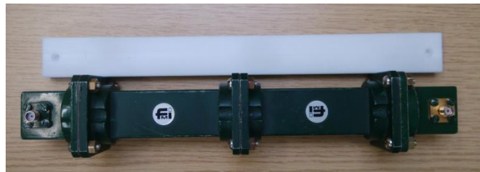
Fig.5.51. WR-90 waveguide with SMA connectors and PTFE bar
