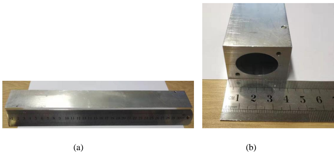
Fig.5.41 Configuration of metallic waveguide: (a) Top view; (b) Front view
