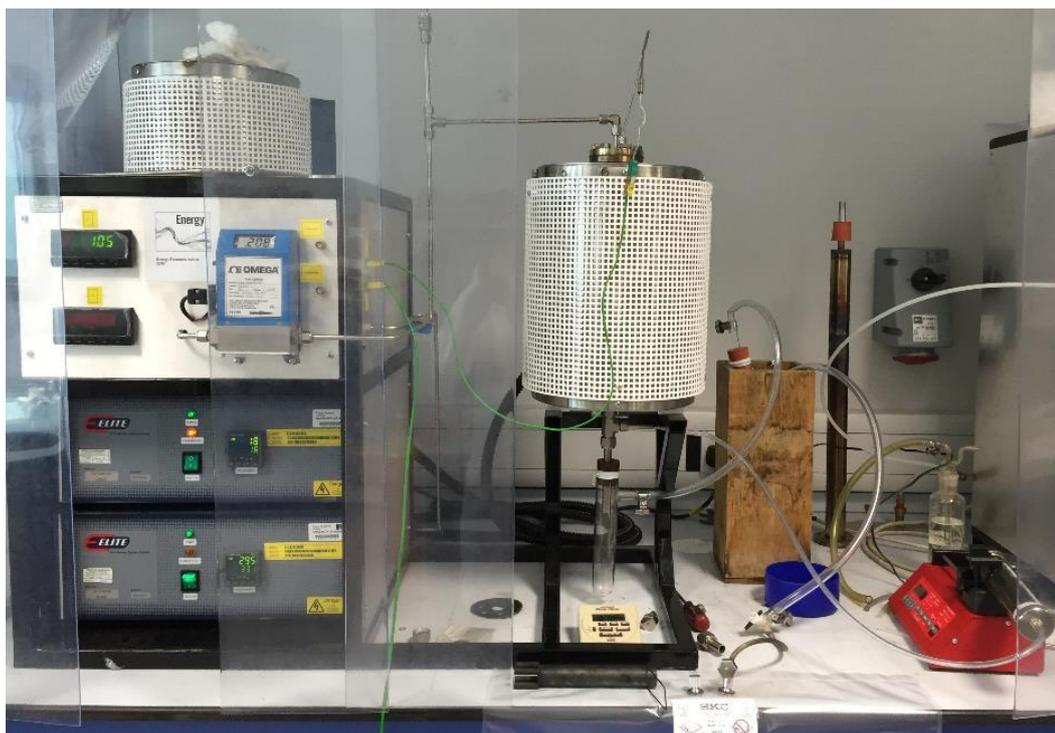
**Figure 3.2-2: Photograph of the pyrolysis system**
