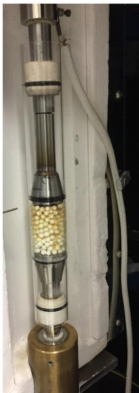
**Figure 3.2-12: Photograph of the packed-bed DBD plasma-catalytic reactor**
