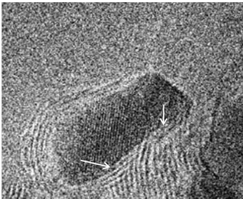
Fig; 2.9 19 ; HRTEM image of the catalyst nanoparticles during the in-situ CNTs growth process, the arrows show the mono-atomic steps in the catalyst nanoparticle, where the carbon atoms diffuse through and form a CNT.
