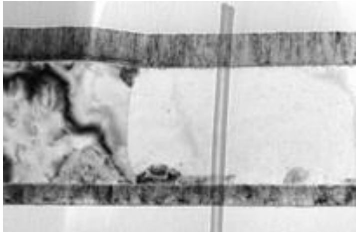
Figure 2.17 Hydrocarbon contamination deposited after a STEM line-scan, seen as the vertical line passing down the image (81).
