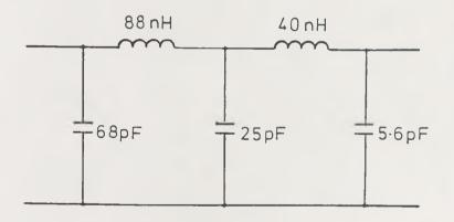
V.H.F. Linear Phase L.P.F.  $f_0 = 100 \text{ MHz}$
