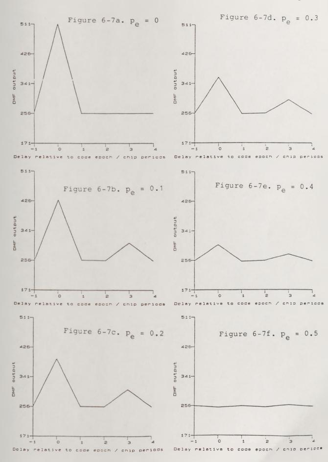
Figure 6-7. DMF mean output against delay with delayed path 6 dB below main path.
