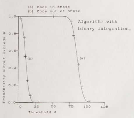
Figure 6-13. Probability algorithm exceeds threshold output.  $p_{\rm e} = 0.3274 \,, \; E_{\bar{\rm c}}/N_{_{\rm O}} = -10 \; {\rm dBs} \,.$
