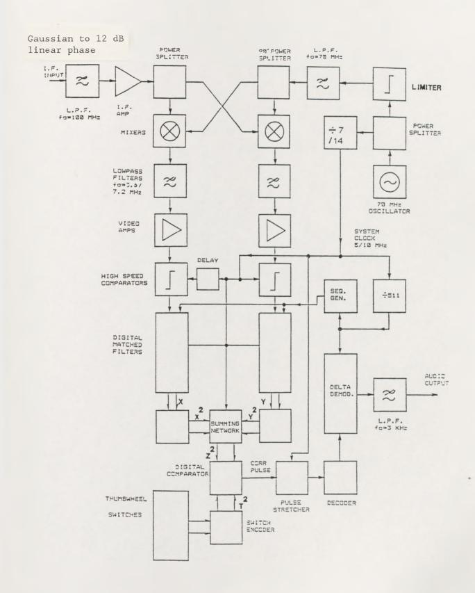
Figure 5-10. Practical DSSS receiver block diagram
