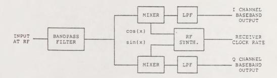
Figure 4-18. DSSS Receiver RF down conversion section.
