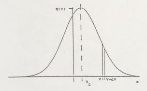
Figure 2-7. Gaussian probability density function.
