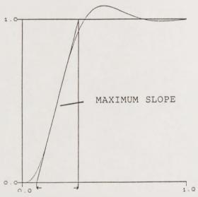
Figure 3-6b. Risetime by maximum slope definition.
