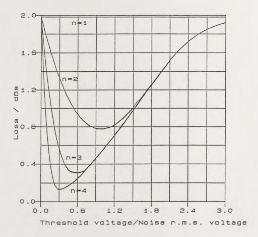
Figure 2-17. Effect of quantization threshold on processing gain loss for constant input snr.
