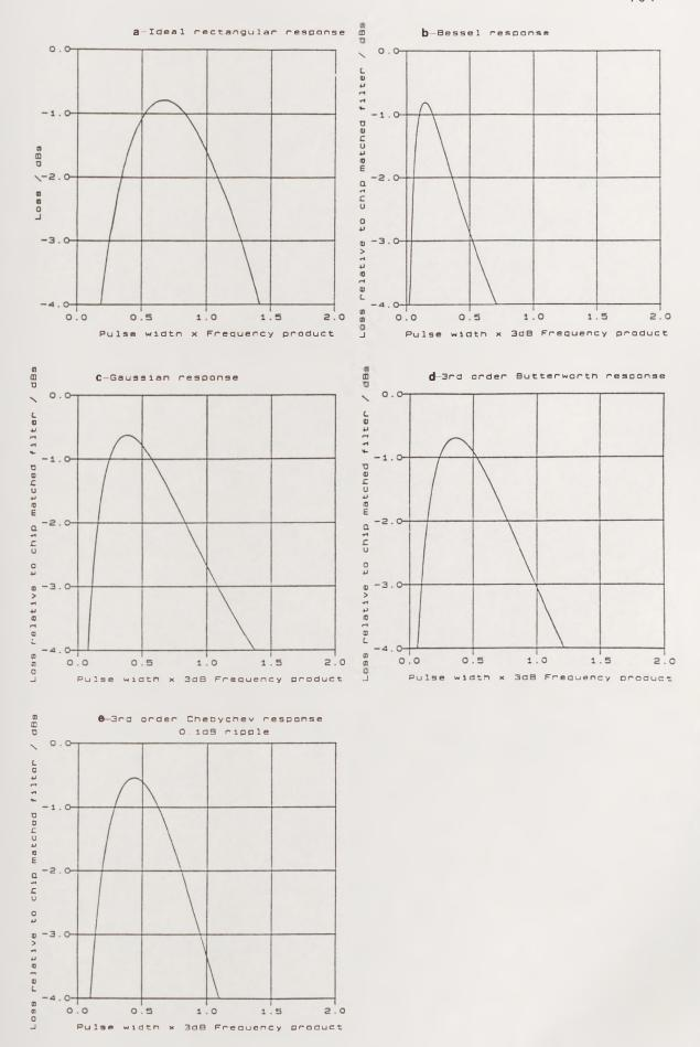
Figure 3-5. Loss relative to ideal chip matched filter for test filters.
