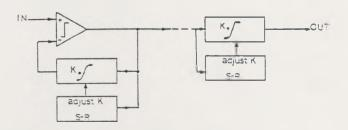
Figure 5-5b. Continuously variable slope delta modulator/demodulator block diagram.
