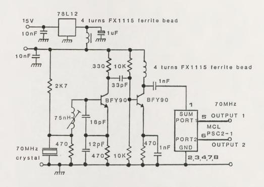
Figure 5-2. 70 MHz oscillator.
