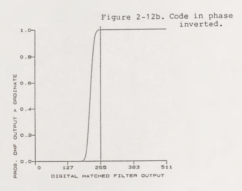
Figure 2-12. Cumulative PDF of DMF output.
