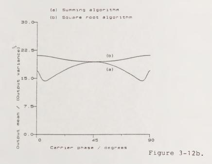
Figure 3-12. Output statistics for algorithms,  $V/\sigma = 1.0$ .
