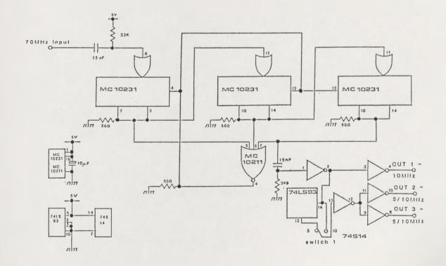
Figure 5-3. 70 MHz divider and system clock generator.
