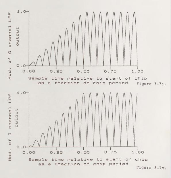
Figure 3-7. Lowpass filter risetime superimposed on mixer output null pattern.
