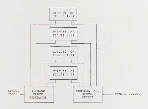
Figure 4-15. Code Synchronization Detection by 4 Single Threshold Crossing Detectors with Binary Integration.
