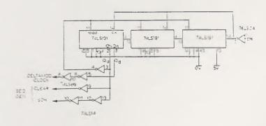
Figure 5-7. CVSD clock and synchronization generator.
