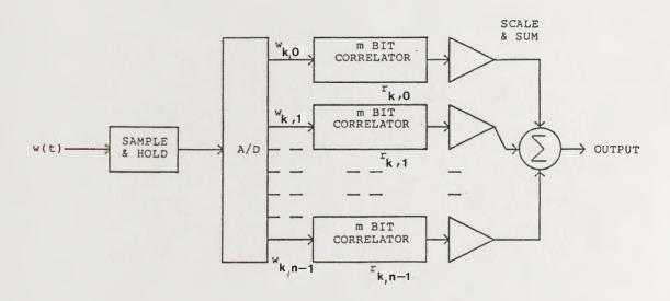
Figure 2-2. m by n bit Digital Correlator.
