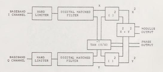
Figure 4-19. DSSS Receiver baseband section.
