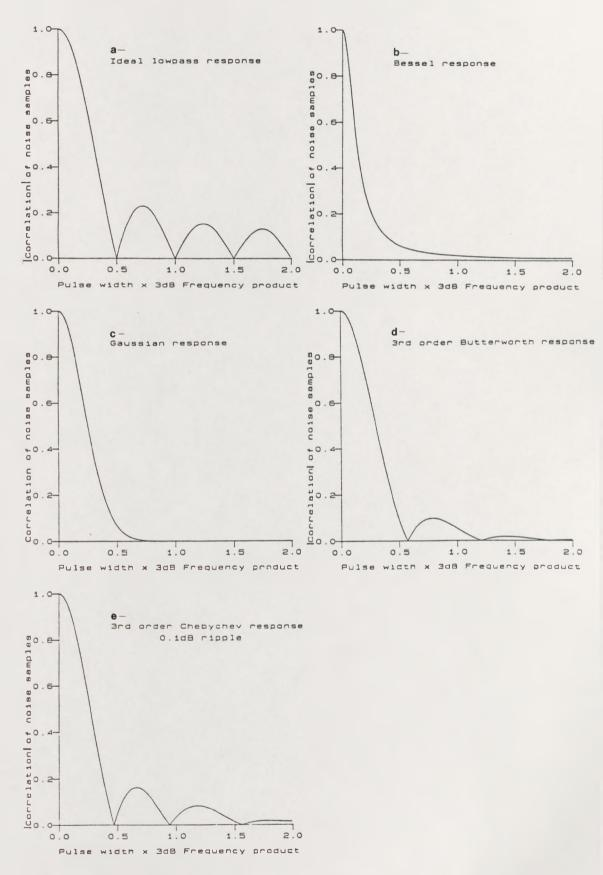
Figure 3-3. Modulus of correlation of lowpass noise samples for test filters.
