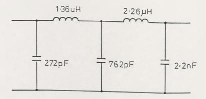
Figure 5-12. Baseband lowpass filter.
