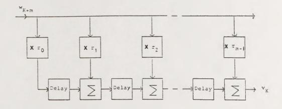
Figure 2-4. Binary Correlator with pipelined adders
