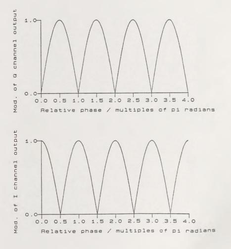
Figure 3-2. Modulus of I and Q channel outputs with varying relative RF carrier phase.
