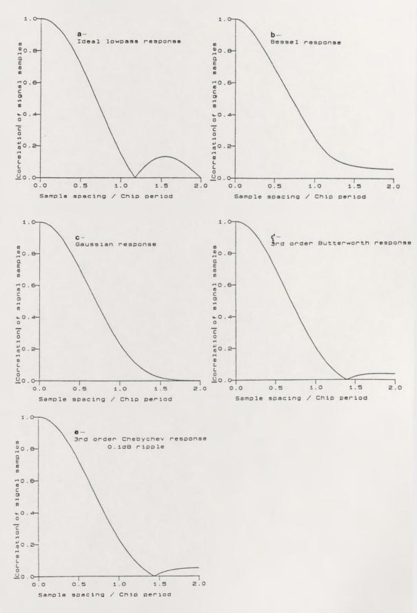
Figure 3-4. Modulus of correlation of lowpass signal samples for test filters.
