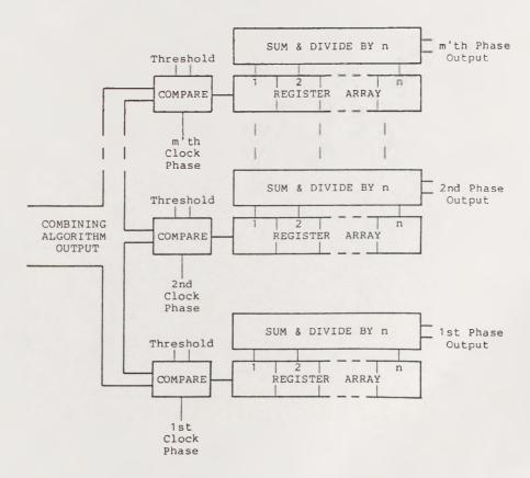
Figure 4-12. Production of Sum of Threshold Crossings.
