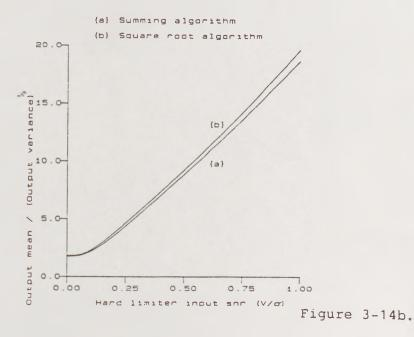
Figure 3-14. Output statistics for algorithms, increasing snr, constant phase(45°)
