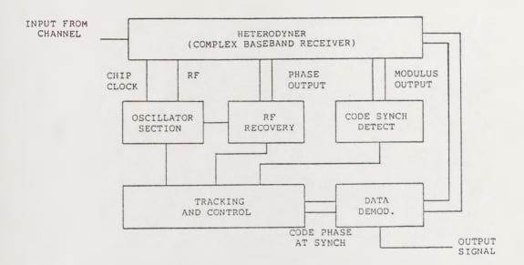
Figure 4-17. DSSS Receiver block diagram.
