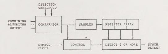
Figure 4-14. Code Synchronization Detection by Single Threshold Crossing with Binary Integration.
