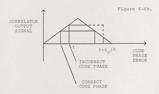
Figure 4-6a. Dither loop. Figure 4-6b. Error signal.
