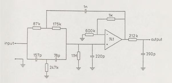
Figure 5-20. CVSD demodulator audio lowpass filter.
