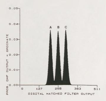
Figure 2-16. DMF output PDF for code in phase and noise only cases.
