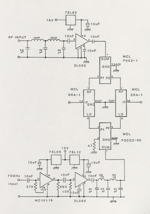
Figure 5-11. Receiver input filter and complex baseband converter.
