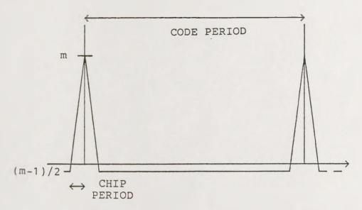
Figure 2-13. Autocorrelation function of practical code for optimum detection.
