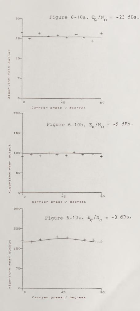
Figure 6-10. Square root algorithm mean output against relative carrier phase.
