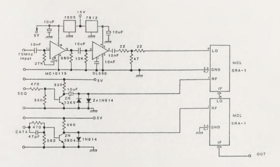
Figure 5-8. Transmitter IF modulator section.
