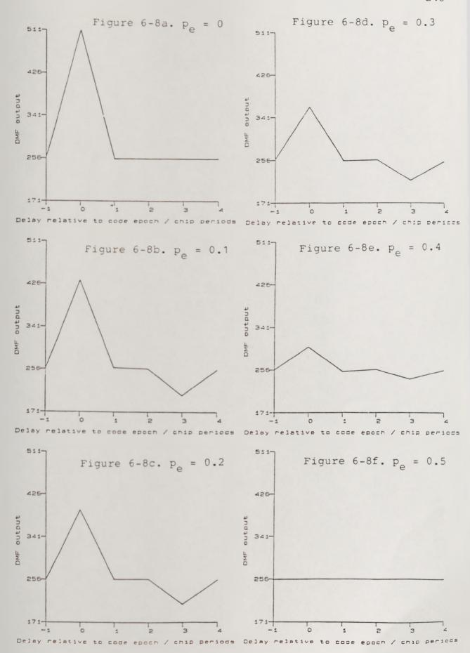
Figure 6-8. DMF mean output against delay with delayed path 6 dB below main path.
