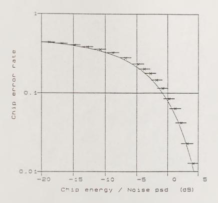
Figure 6-2. Measured chip error rate.
