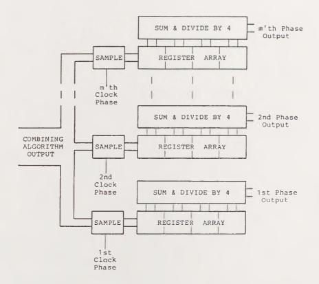
Figure 4-11. Production of Average Algorithm Output.
