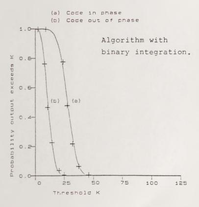
Figure 6-11. Probability algorithm exceeds threshold output.  $p_e = 0.4437$ ,  $E_c/N_o = -20$  dBs.
