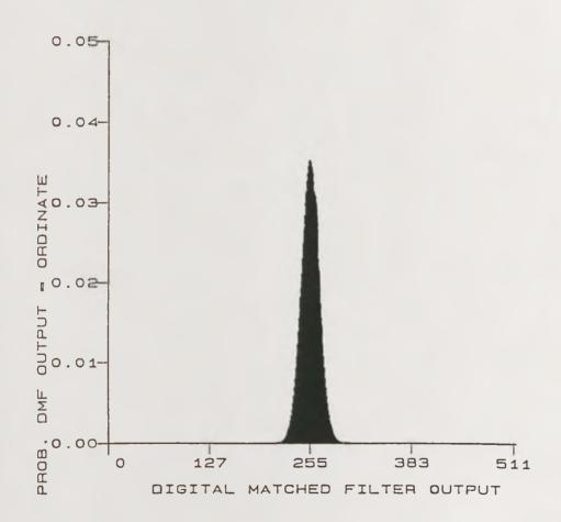
Figure 2-14. DMF output PDF, noise only case.
