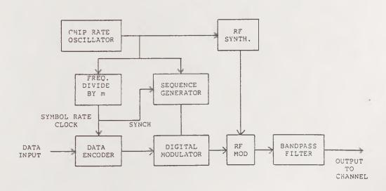
Figure 4-16. DSSS Transmitter block diagram
