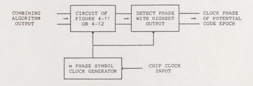
Figure 4-13. Code Epoch Detection.
