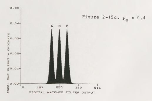
Figure 2-15. DMF output PDF for code in phase and code out of phase cases.
