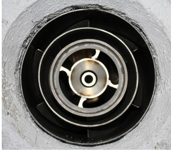
Figure 4.15: A photograph of the front of the scale down version of the Doosan Babcock burner [140, 176].
