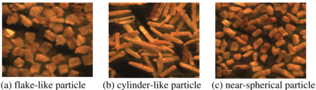
Figure 3.2: Images of the hardwood sawdust particles with flake-like (a), cylinder-like (b), and near-spherical (c) shapes. [79].
