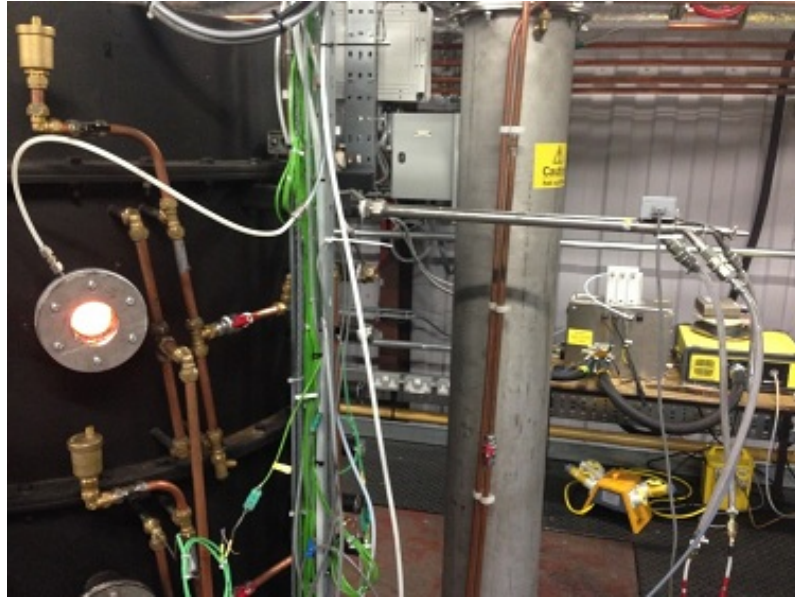
Figure 4.8: Photograph of the suction pyrometer during temperature measurements - Suction pyrometer positioned in the first 38.1 mm measurement port during an air-fired experiment [176].
