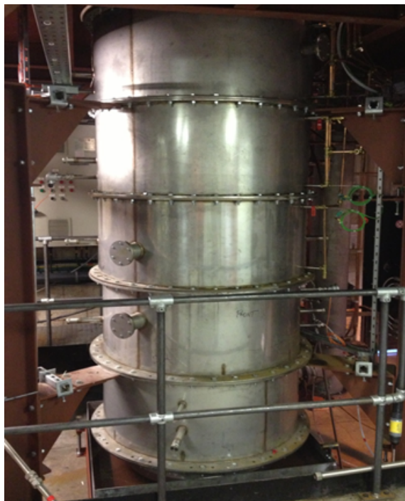
Figure 4.7: Photograph of the lower sections of the PACT Combustion Rig [176].
