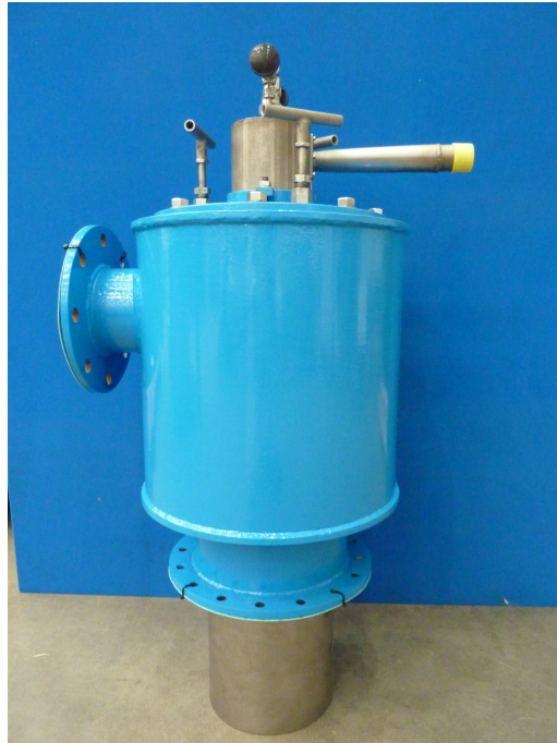
Figure 4.13: Photograph of an outer view of the burner before being applied to the furnace [140, 176].
