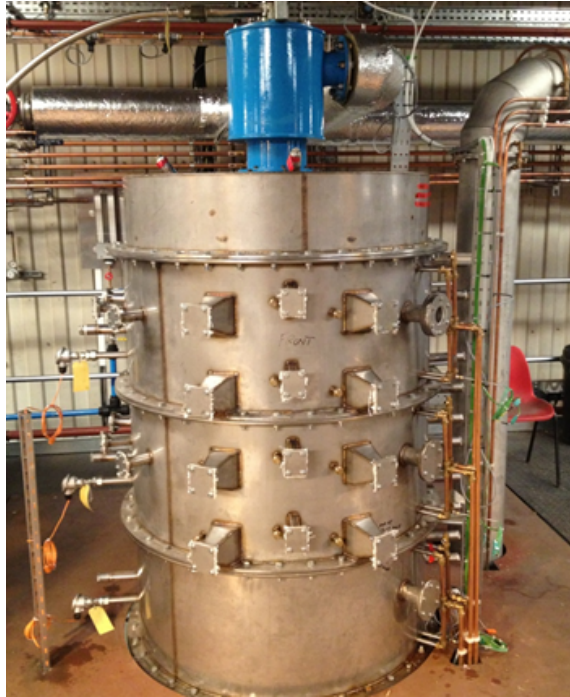
Figure 4.6: Upper sections of the PACT Combustion Rig with viewing ports and burner on the top [176].
