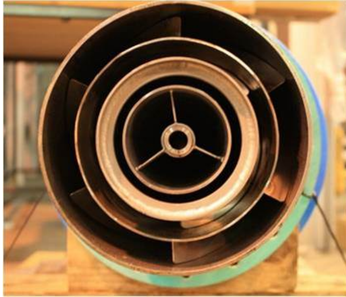
Figure 4.21: A photograph of the front of the Doosan Babcock biomass burner.
