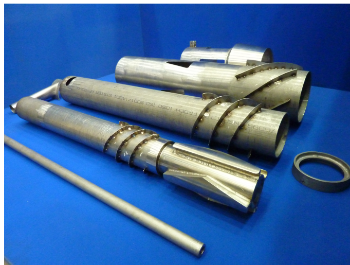
Figure 4.14: Photograph of the primary, secondary and tertiary inlets of the burner [140, 176].
