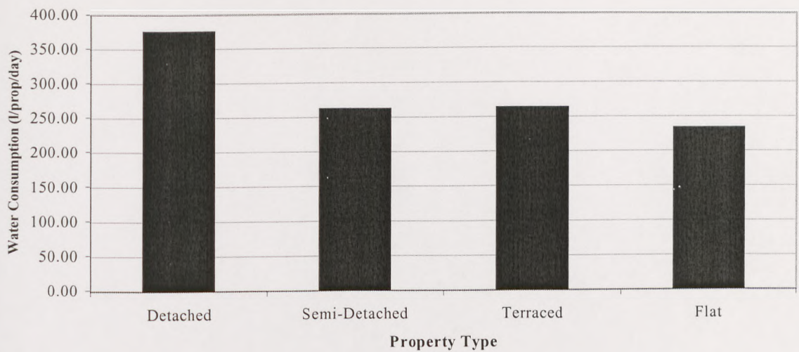
Figure 5.26: Average per property water consumption for one-person households in the Thames Water study
