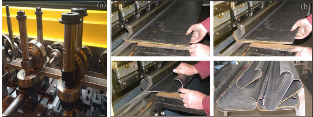
Fig. 2.1. Manufacturing process of CFS elements using (a) rolling (Tsang et al., 2018), or (b) press-braking (Bagheri Sabbagh et al., 2011)
