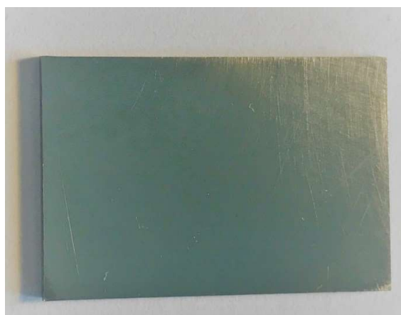
Figure 2.2: Stainless steel 316L after polishing.
