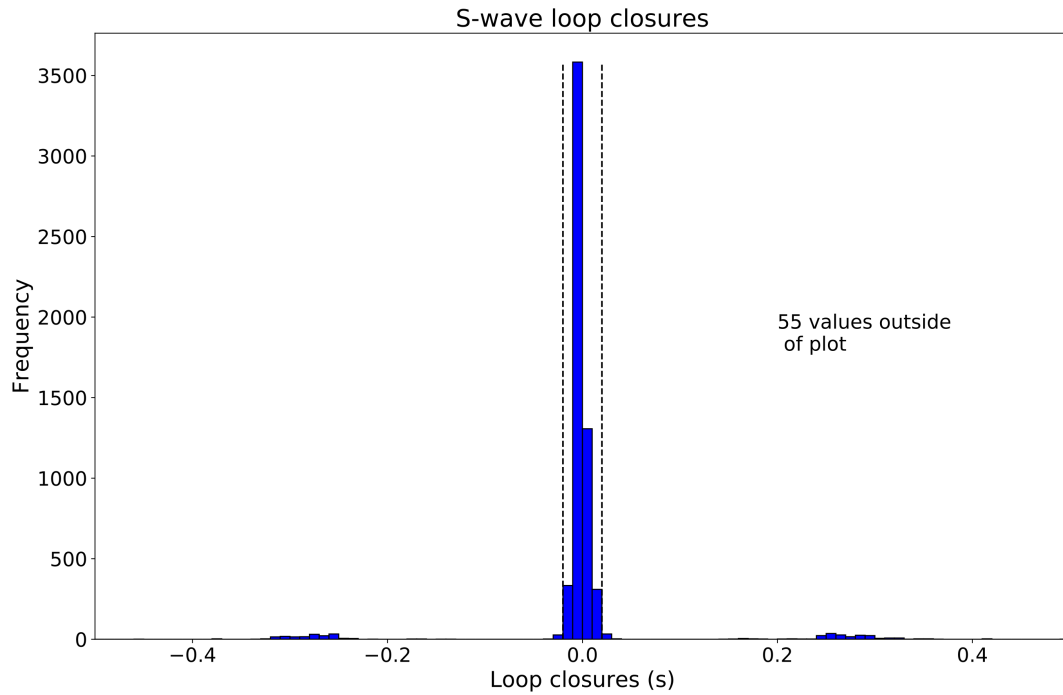
Figure B.3: Histogram of loop closures for the results of the S wave analysis on the aftershocks of the El Mayor-Cucapah earthquake. The dashed black lines indicate a 0.02 s limit. Some values have been excluded from the plot.
