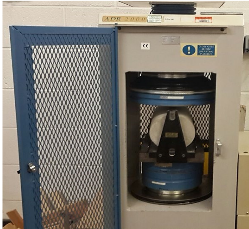
Figure 3-17. Splitting tensile strength test
