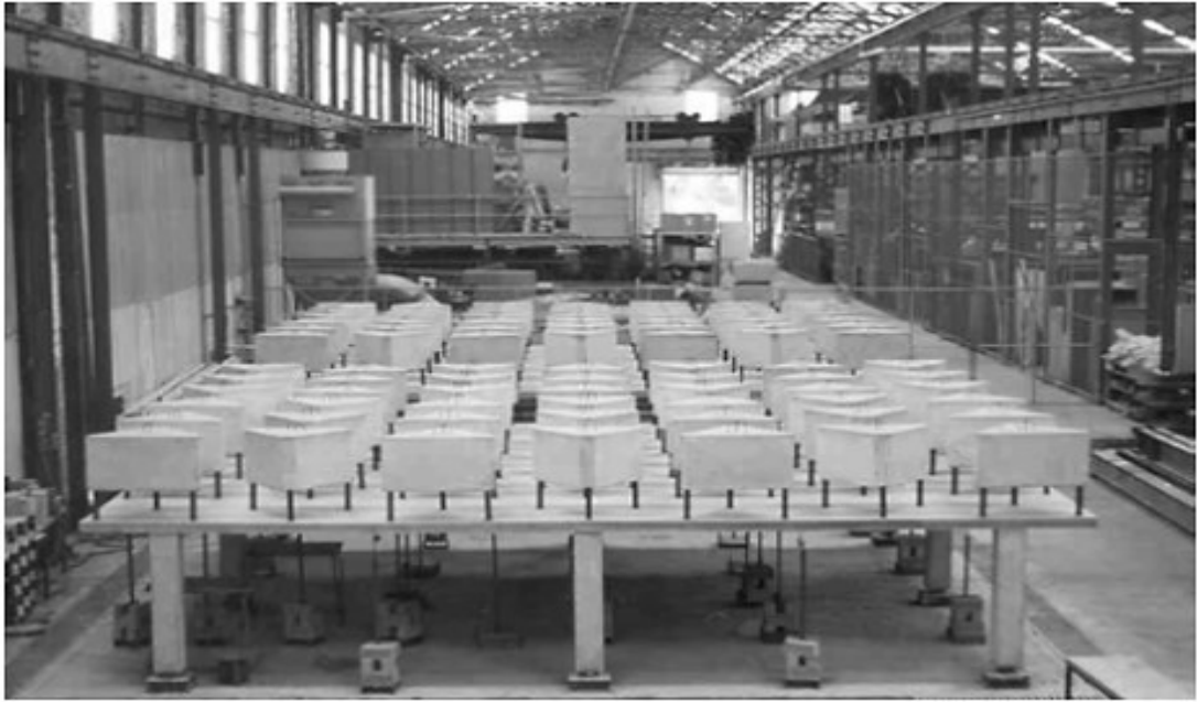
Figure 2-44. Reinforced concrete (RC) flat slabs under tests (Gilbert & Guo, 2005)
