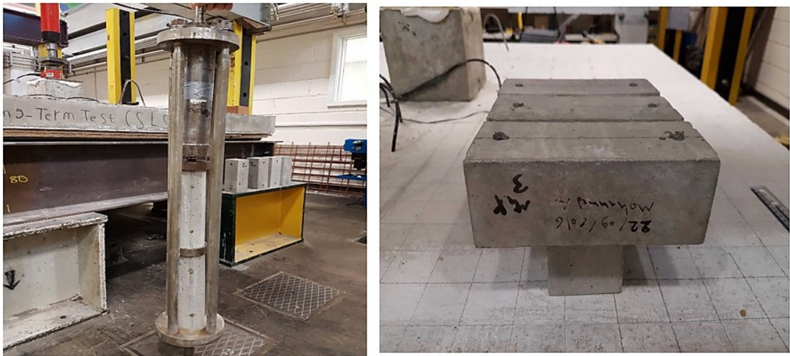
Figure 3-13. Creep and shrinkage small specimens
