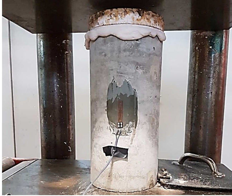
Figure 3-16. Modulus of elasticity test of cylinder
