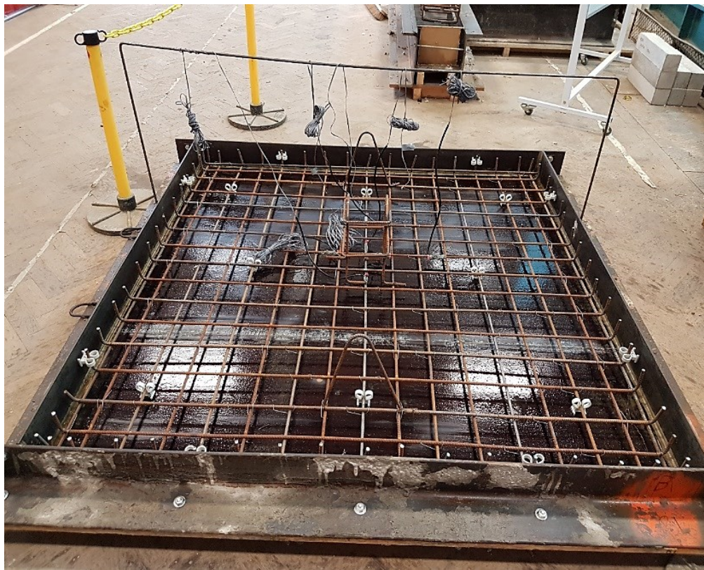
Figure 3-10. Arrangements of reinforcement bars
