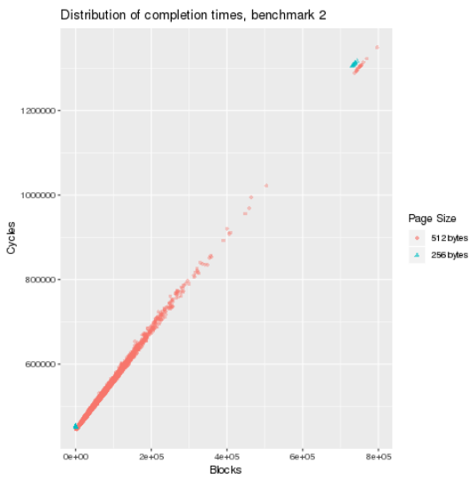
Figure 5.30: The range of completion times for benchmark 2 with 512-byte and 256-byte partial paging
