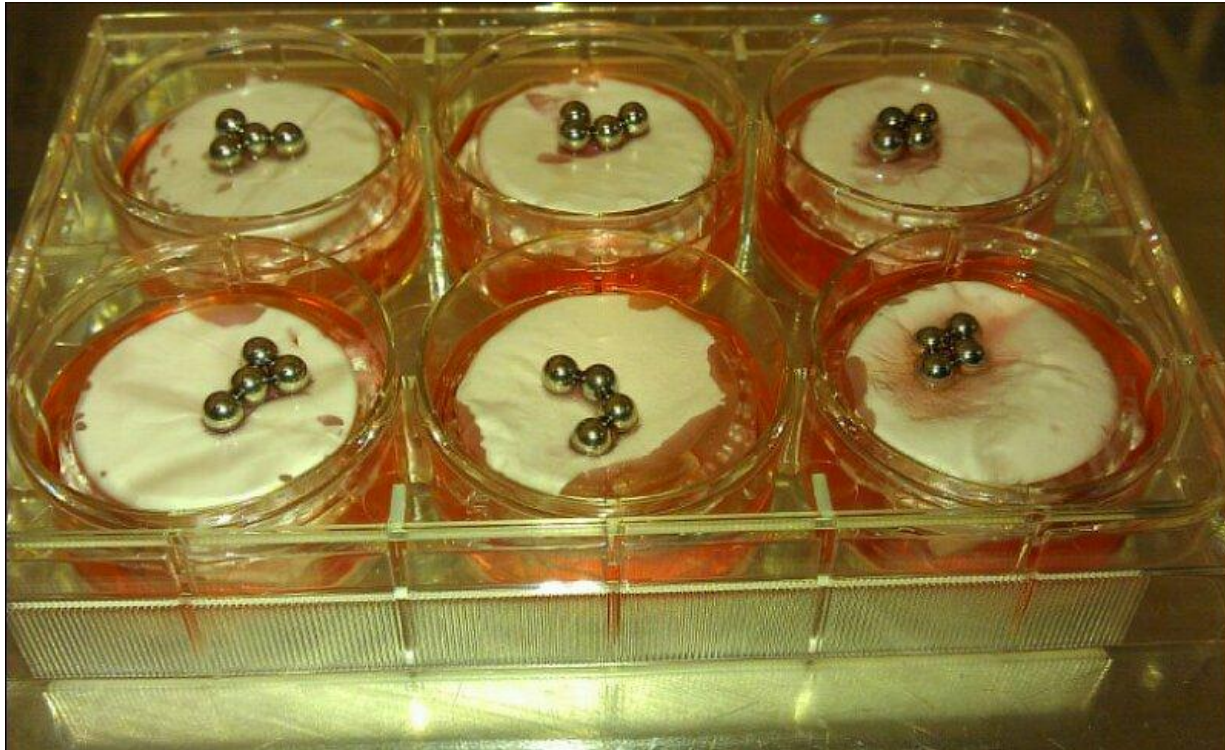
Fig 2.11.1. Variable stress rig (1) utilising inverted Scaffdex™ rings in a six well culture plate with four ball bearings used to vary stress on alternate days.
