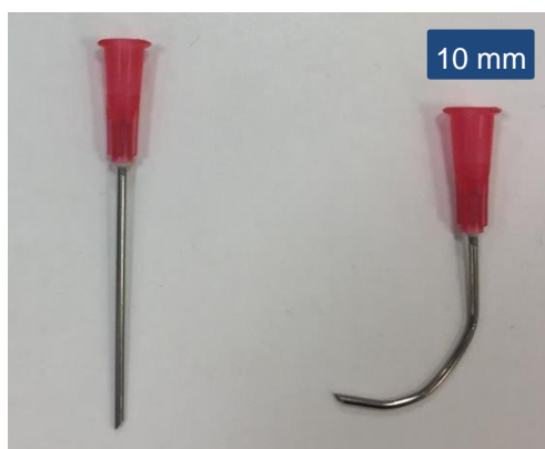
Figure 3-10 Syringes used for water in oil and oil in water contact angle measurements
