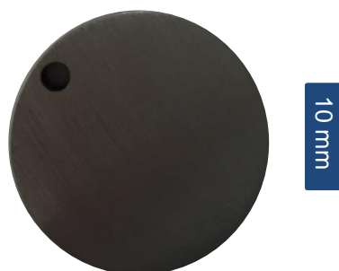
Figure 3-1 X65 carbon steel mass loss specimen
