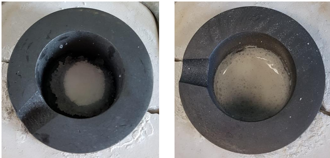
Figure 14. Solar salt mixture when the graphite crucible is placed in the furnace. (Left) pure salt being melted; (Right) nanofluid with 1 wt. % \text{Al}_2\text{O}_3 nanoparticles fully melted.
