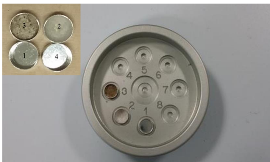
Figure 38. DSC testing disc with 3 samples numbered on the tray as: 1) Empty pan used as a main reference; 2) NaNO 3 sample; 3) KNO 3 sample. The four pans at the corner of the figure are the same sample, with an extra empty pan number-4 used inside the DSC reference compartment.
