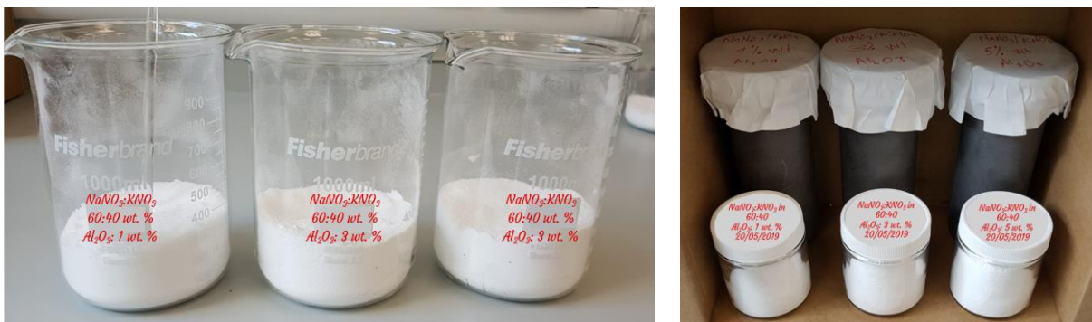
Figure 13. Example of binary nitrate salt doped with alumina nanoparticles ( \text{Al}_2\text{O}_3 , 80% alpha / 20% gamma, 99.9% pure, d_p = 50 \text{ nm} ) samples produced using the dry mixing process (1 wt. %; 3 wt. % and 5 wt. % from left to right, respectively). (Left) In this particular case, glass jars were used to mix a total amount of 350 g solar salt per batch, each consisting of 210 g of \text{NaNO}_3 and 140 g of \text{KNO}_3 . (Right) samples kept in labelled glass jars.
