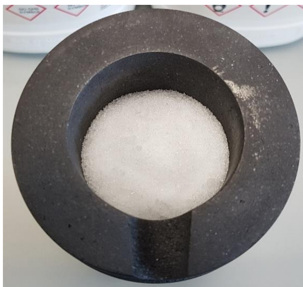
Figure 12. Nitrate salt mixture consisting of 60 wt. % sodium nitrate ( \text{NaNO}_3 ) and 40 wt. % potassium nitrate ( \text{KNO}_3 ), known as “Solar Salt” placed in a graphite furnace crucible.
