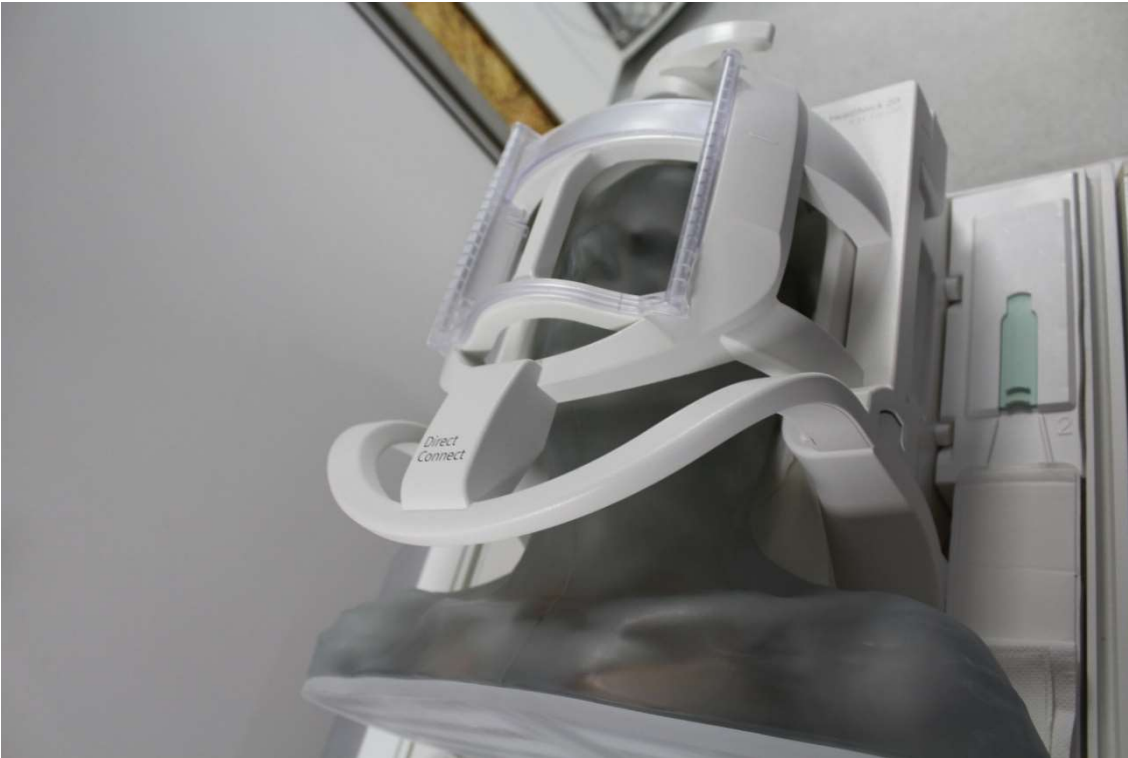
Figure 6-17 The prototype phantom set-up within the MRI head coil. A coil array was also added later to cover the shoulder section of the phantom.
