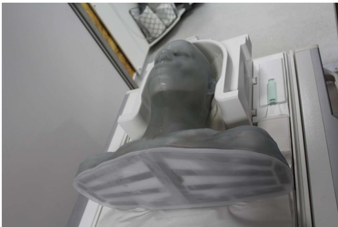
Figure 6-16 Photograph of the phantom, showing the inferior section which is sealed in this prototype.
