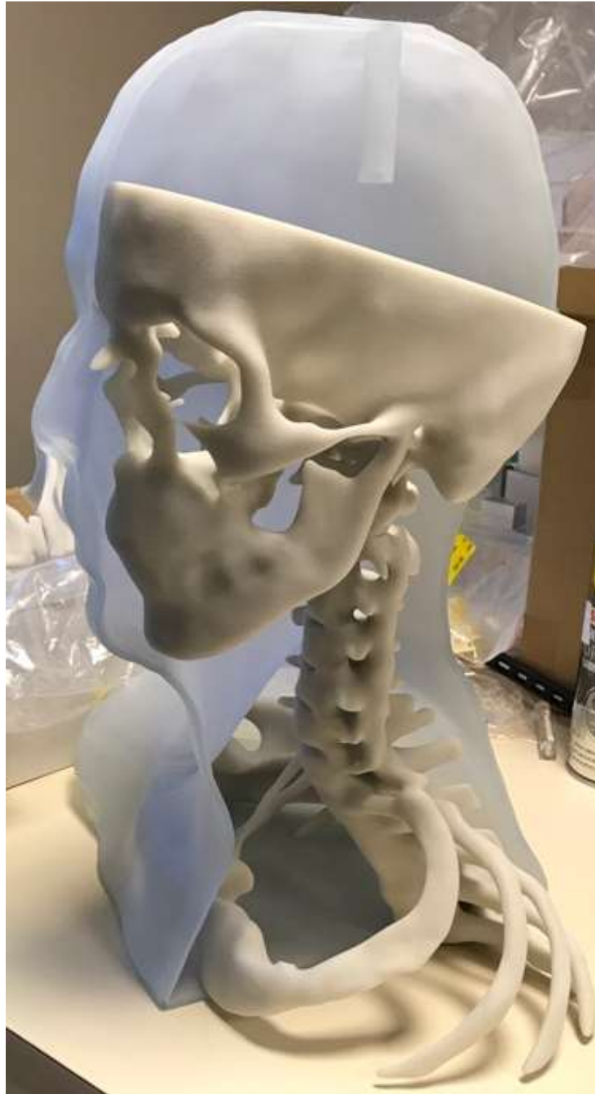
Figure 6-14 The phantom under construction. Half of the outer casing can be seen. The inferior part of the skeleton is also present within the casing. The top section will be attached once the brain is fitted. A cavity in the superior section of the outer casing where a dosimetric chamber could be inserted can be seen. No filling caps are present in positions where the MRI coils would be used.
