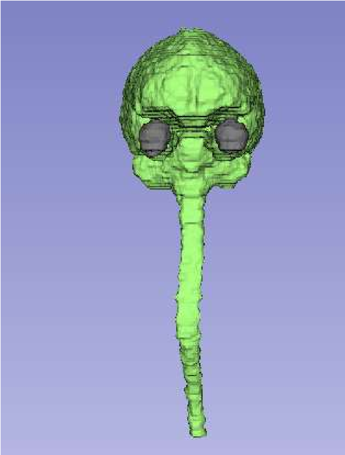
Figure 6-12 Image of the 3D structure mesh which was created as a basis for the brain, brainstem and spinal cord (in green) and the eyes (in grey) in the phantom (coronal view).
