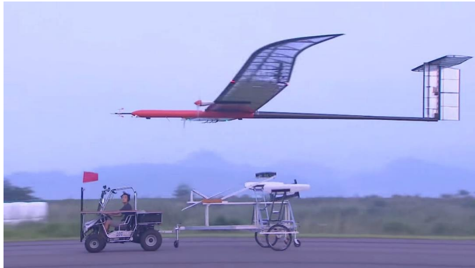
Figure 2-2 EAV-3 takes off with assisted from its trailer at Korean Airport (Directly reproduced from [45]).
