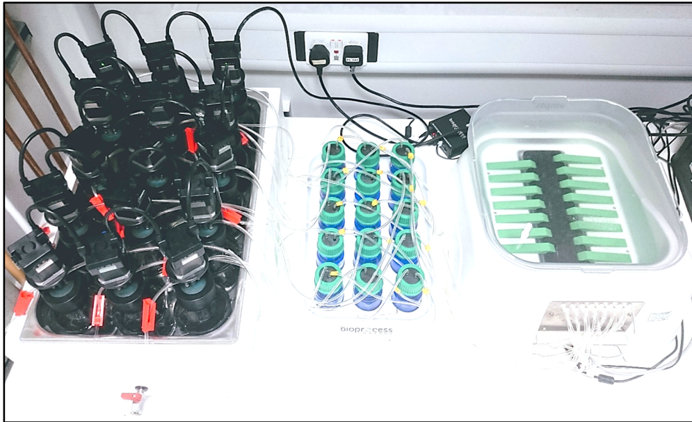
Figure 14. Biochemical methane potential test apparatus set-up.
