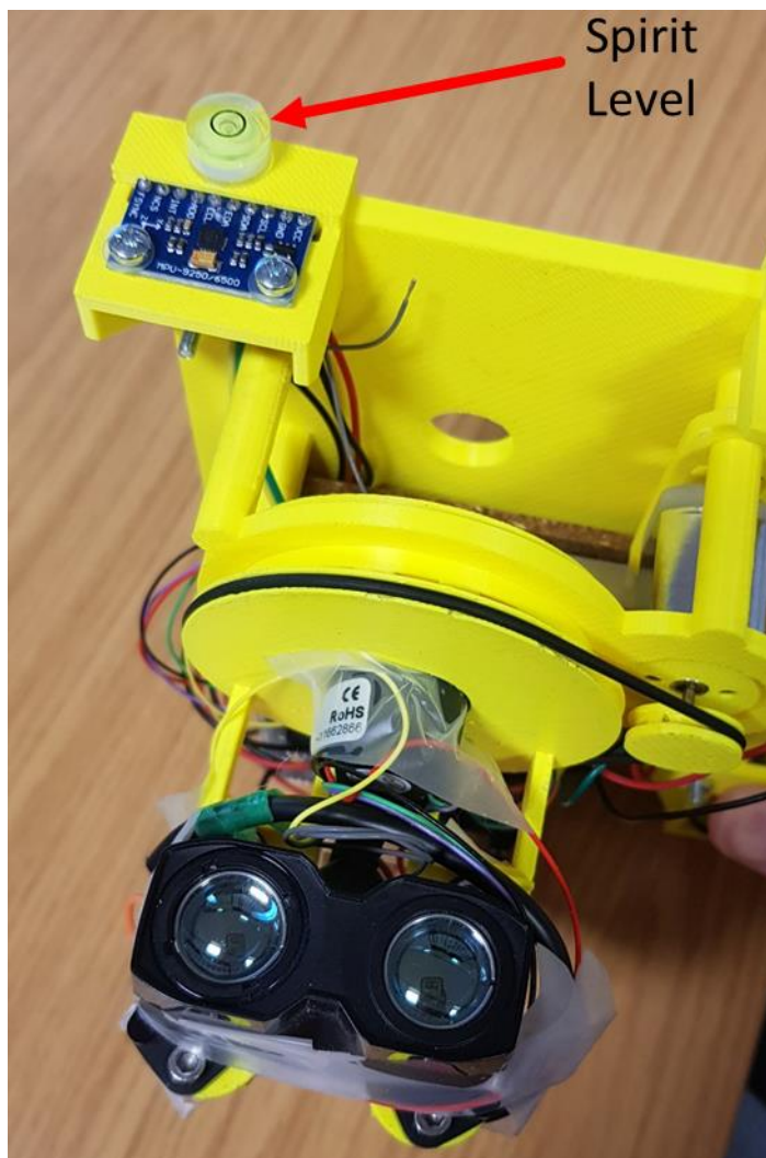
Appendix Figure H.1. Prototype in vertical orientation with MPU9250 and spirit level dot
