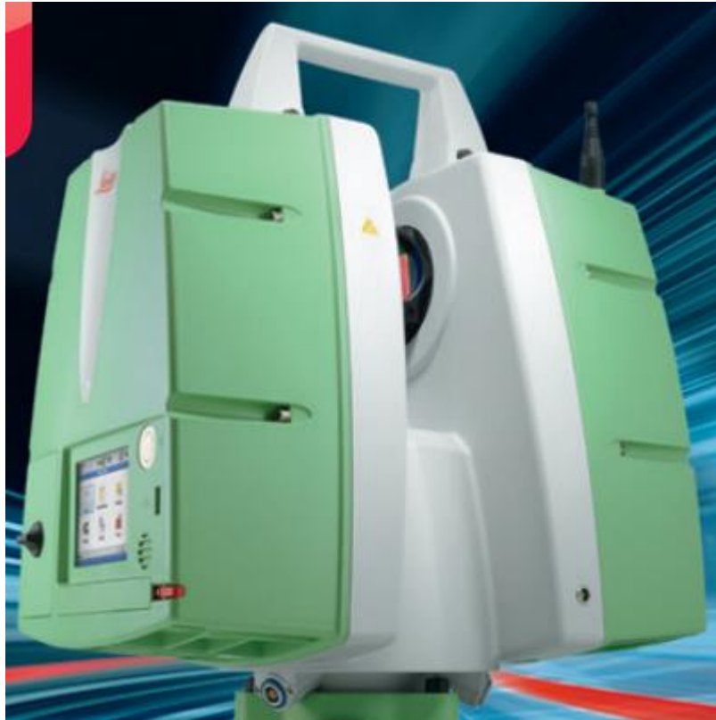
Figure 4.2. Leica Scanstation P20 [150]
