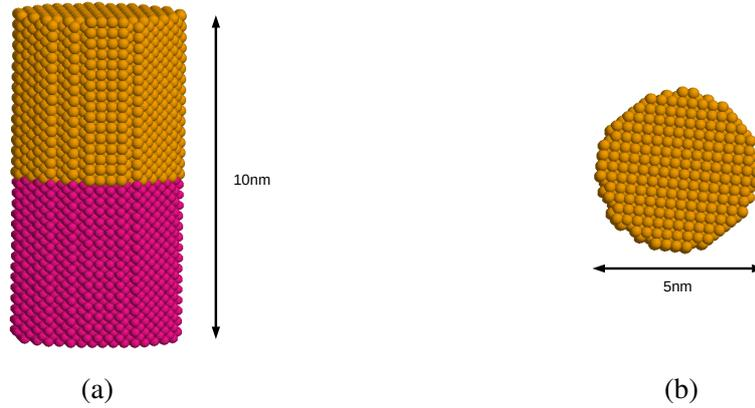
Fig. 4.1 A 3D image of exchange-coupled composite (ECC) media. Figure (a) shows a profile picture of the grain which comprises two magnetic phases suggested by different colors. The magenta color on the bottom of the grain represents FePt with 5nm height and the yellow color represents the soft Fe phase. On image (b) it is illustrated a top view of the ECC grain.
