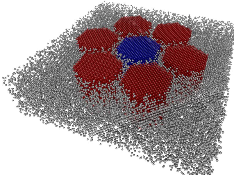
Fig. 3.7 A typical configuration system of the hexagonal distribution of the grains with an inter-layer doping constant of 30%. Each grain is hexagonal-based with a corner-to-corner diameter of 5 nm and 5 nm height.
