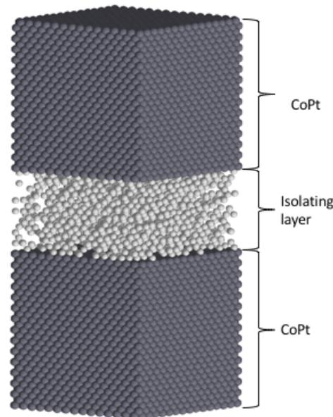
Fig. 3.3 A visualisation of the bilayer system made of two identical ferromagnets separated by a dilute oxide layer with a doping concentration of 30% of magnetic atoms in this case. The width and height of each ferromagnet are 5 nm.
