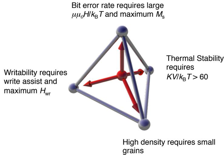
Fig. 1.3 Illustration of *quadrilemma* of heat-assisted magnetic recording. This picture has been taken from reference [28].
