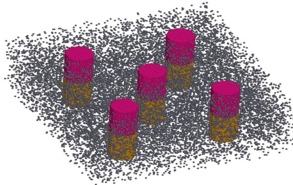
Fig. 3.13 A visualisation of a complex structure of 5 ECC grains coupled by a non-magnetic layer with a doping density of 15%.
