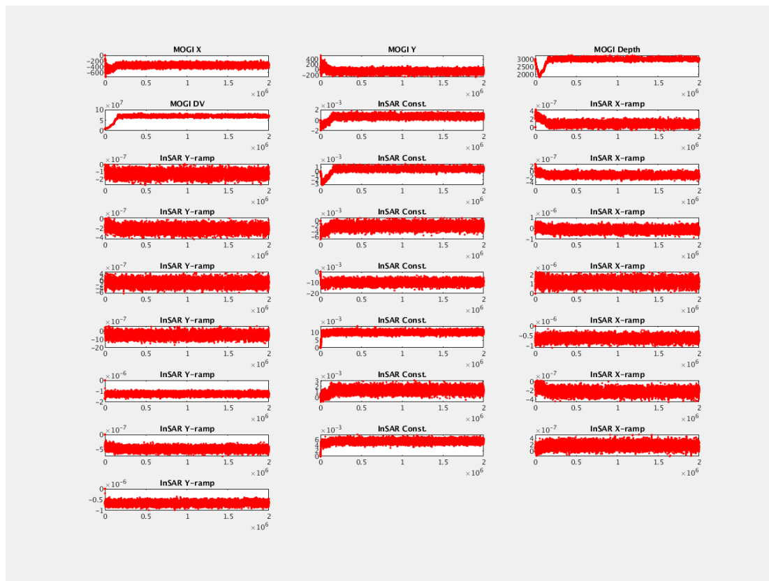
Figure A.40: Accepted parameter solution (each plot) against iterations, for the inversion that I carried out using LOS velocities over the 15-year long InSAR time-series, assuming a Mogi source and solving its location (X,Y), depth, volume change (DV), as well as for constants estimating the deformation at the reference, and possible ramps along X and Y.
