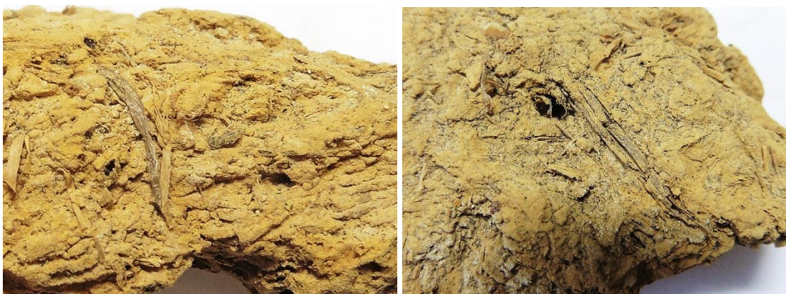
Plates No. 5 & 6: The above plates show fractured surfaces in which the abundance of fibre can be seen, with straw and grass stalks both apparent.
