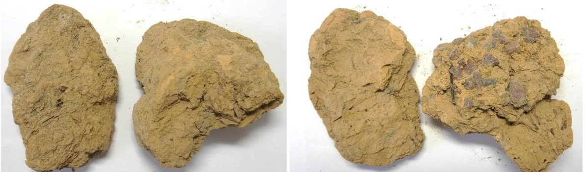
Plates No. 1 & 2: The above plates show the intact pieces of mortar as received, with the left plate showing one of the larger surfaces of the intact pieces, with the right plate showing the opposite face. Note the presence of a crushed aggregate chips in the surface of one fragment (right piece).
