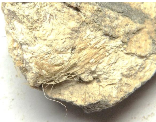
Plates No. 4 & 5: The above plates show fractured surfaces in which an abundance of fibre can be seen, with hair fibre occurring as clumps, poorly separated fibres, and as individual hair fibres. The hair ranged in colour from white, light and dark brown to red, with the fibres being of animal hair, possibly horse body hair.
