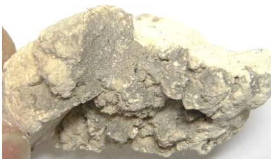
Plates No. 2 & 3: The left plate shows a close-up of a soiled surface within a void in the mortar, where water percolation with the deposition of both transported debris and redeposited leached lime were both apparent. The right plate shows a freshly fractured surface through the thickness of the pointing, with “aggregates” apparent along with lime inclusions and hair fibres. Tests on the fractured surfaces with a phenolphthalein indicator solution confirmed that the mortar was fully carbonated.
