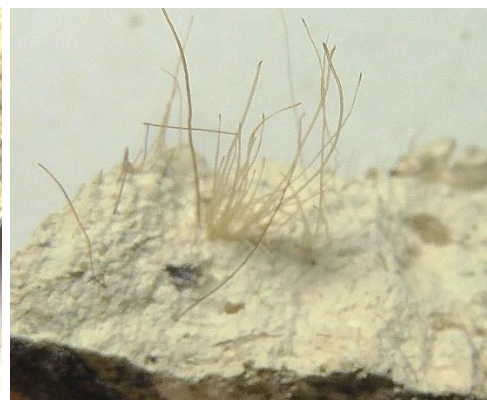
Plates No. 4 & 5: The above plates show fractured surfaces in which an abundance of fibre can be seen, with hair fibre occurring as clumps, poorly separated fibres, and as individual hair fibres. The hair ranged in colour from white, light and dark brown to red, with the fibres being of animal hair, possibly horse body hair.
