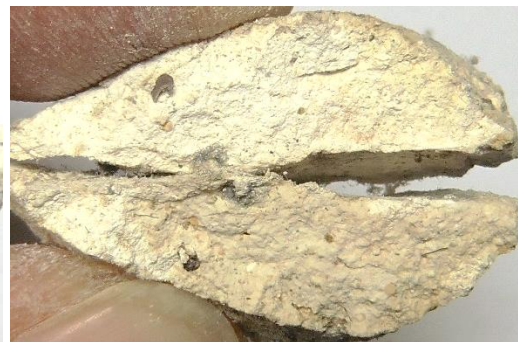
Plates No. 2 & 3: The left plate shows a close-up of a soiled surface within a void in the mortar, where water percolation with the deposition of both transported debris and redeposited leached lime were both apparent. The right plate shows a freshly fractured surface through the thickness of the pointing, with “aggregates” apparent along with lime inclusions and hair fibres. Tests on the fractured surfaces with a phenolphthalein indicator solution confirmed that the mortar was fully carbonated.
