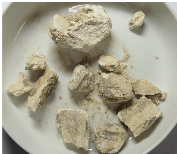
Plate No. 1: The above plate shows the intact pieces of mortar as received, which was found to consist of twelve mortar fragments and a small quantity of fines.
