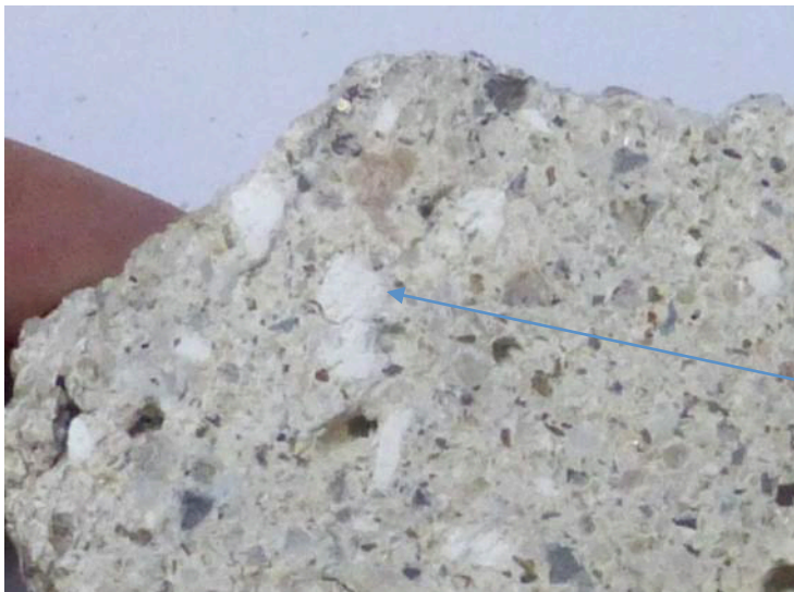
Plate No. 9: Quicklime Binder? Inclusions sub- round, sub-angular and irregular. No – The mortar was mixed in the laboratory from a Hydrated lime.
