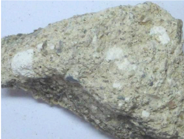
Plate No. 8: Quicklime Binder, where inclusions are angular to sub-angular.
