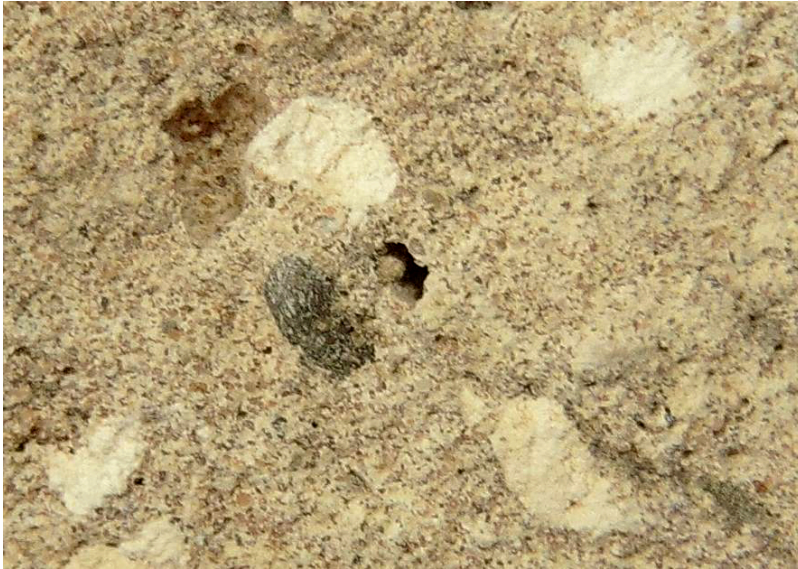
Plate No. 20: Quicklime in a 15 th C Hot Lime Mortar. Thin sections from this sample are shown below
