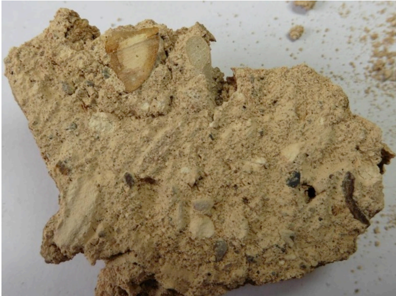
Plate No. 23: Quicklime in a 13 th C Hot Lime Mortar. Thin section from this sample are shown below
