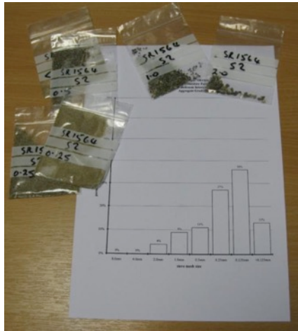
Plates No. 30, 31 & 32: Grading of the aggregate after drying to determine particle size distribution.
