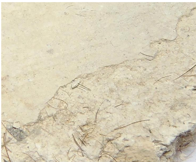
Plates No. 3 & 4: The left plate above is a close-up of a fractured edge, showing the abundance of hair present in the plaster coat. With the right plate being a magnified view of the inner contact surface with retained clay mortar and straw reinforcement from the base coat plaster adhering strongly to the plaster finish coat.
