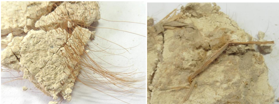
Plates No. 3 & 4: The left plate above is a close-up of a fractured edge, showing the abundance of hair present in the plaster coat. With the right plate being a magnified view of the inner contact surface with retained clay mortar and straw reinforcement from the base coat plaster adhering strongly to the plaster finish coat.
