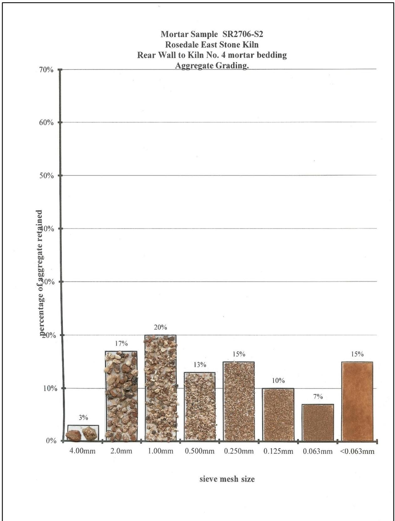
**Figure No. 2** – Aggregate Grading on Aggregate recovered from sample RESK2.
