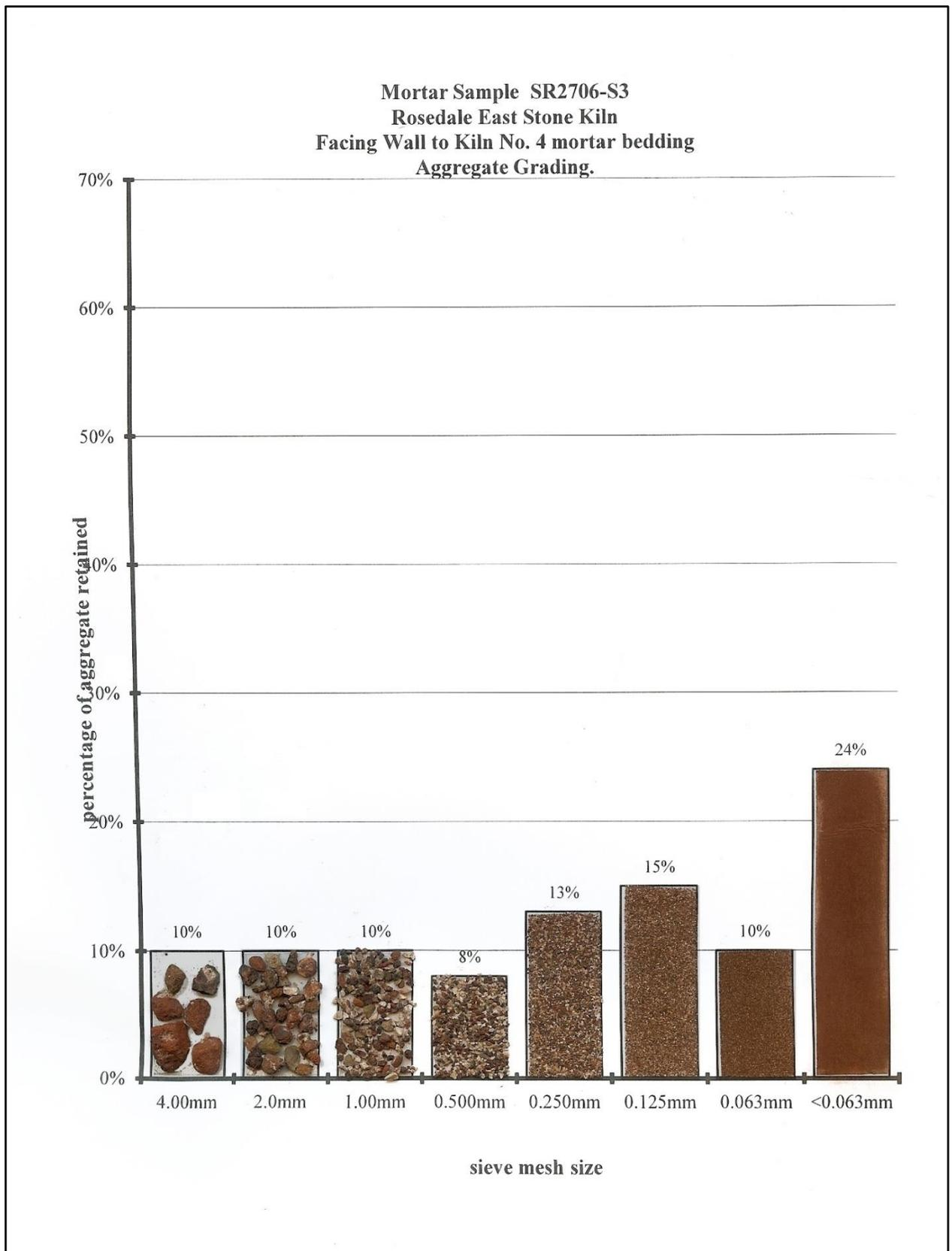
**Figure No. 3** – Aggregate Grading on Aggregate recovered from sample RESK3.
