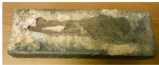
Figure 22: mediaeval brick mortar, Hull; Figure 23: mortared brick from Frank Lloyd Wright house, Chicago, Both mortars slaked to a dry mix and screened.
