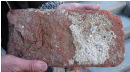
Figure 22: mediaeval brick mortar, Hull; Figure 23: mortared brick from Frank Lloyd Wright house, Chicago, Both mortars slaked to a dry mix and screened.
