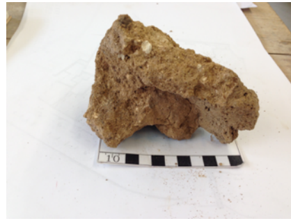
Figure 70 Typical core mortars, Ryton, Malton Figure 71 Lincoln Cathedral Precinct wall
