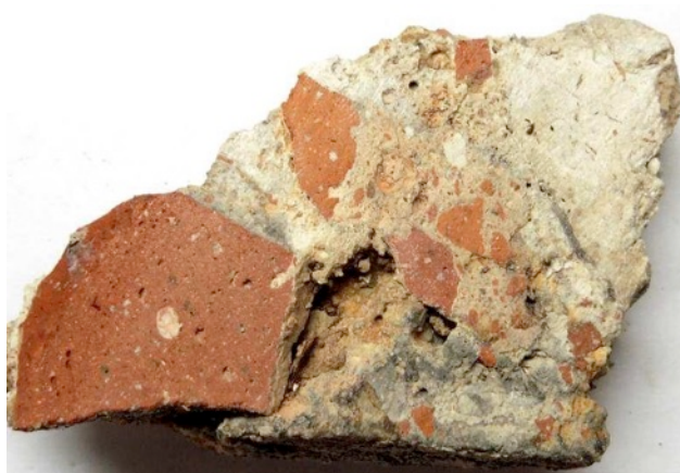
Figure 92. Roman mortar from bath-house at Vindalanda. See Appendix Eleven No.2)
