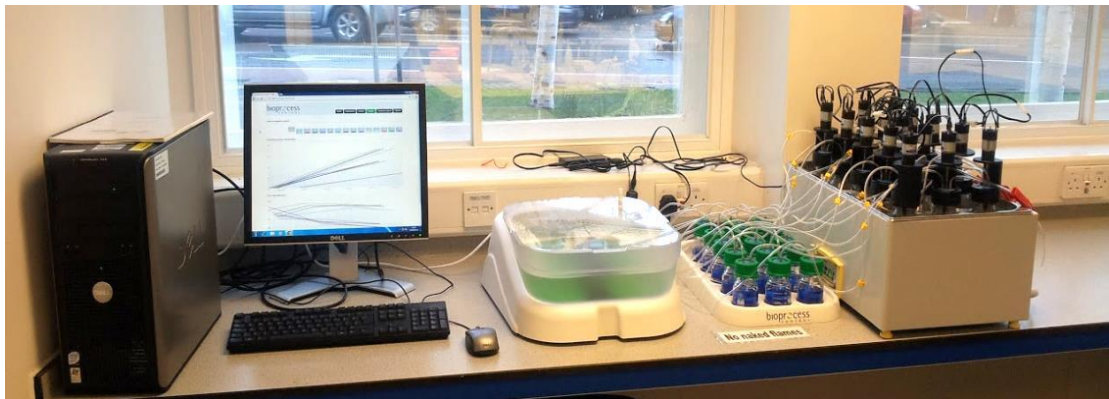
Figure 3.13 Photograph of the batch experimental setup, from the right to left: stirred batch reactors in the water bath, alkaline gas scrubbing systems, the multi-channel volumetric gas meter, and the software user interface [81].
