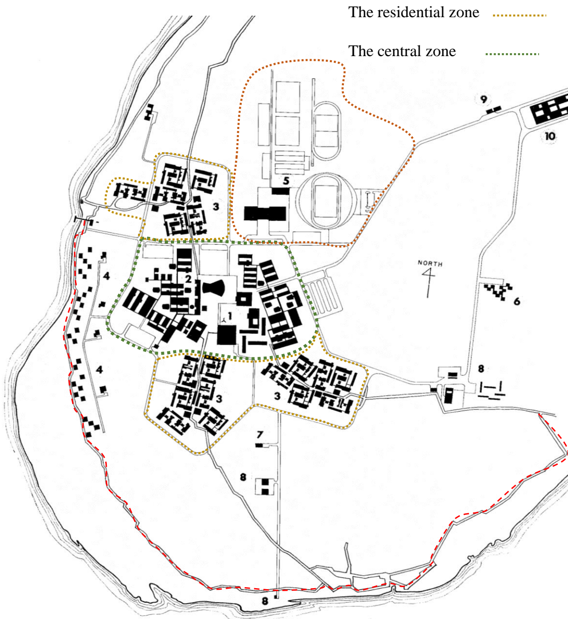
Figure 6-7:: The University site on the shore of the Tigris river is flat except for existing 10- ft high dikes indicated on the plan by heavy irregular red lines. These would determine a change of level within the campus. And the main facilities that are indicated
