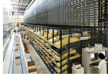
Fig. 2.5 Gravity rack in ware- house
