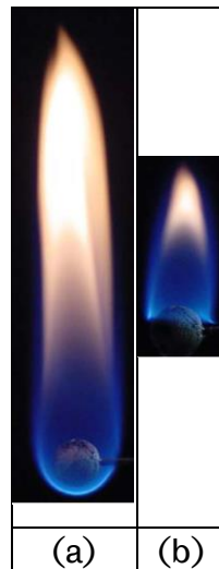
Fig. 2.12 Flame photographs of (a) enveloped flame and (b) Wake flame (taken from [116] with a permission from the publisher)
