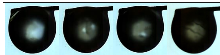
Fig. 6.2 Typical soot contamination from light to heavy surface coverage [97].
