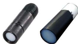
FIG. 5. State-of-art cosine corrector (left) and experimental coupler design D1 (right).
