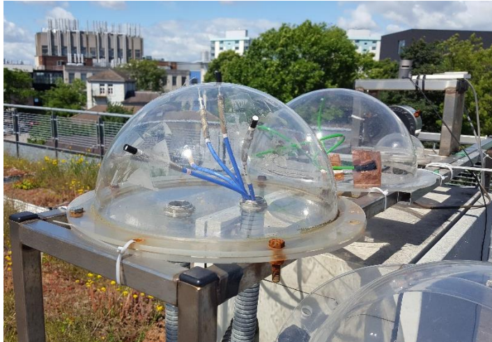
Figure 4.3: Setting of the acquisition station, 5 sensors attached to a semi-spherical acrylic base. Inside the box under the base there was the spectrometer connected to a computer programmed to record the data automatically.
