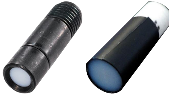
Figure 3.10: Cosine corrector comparison, State-of-Art cosine (left) and CCOC design D1 (right).
