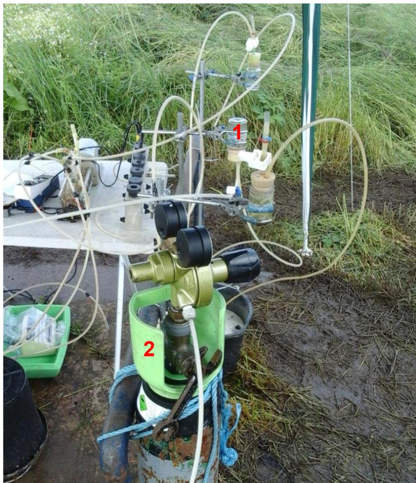
Figure 23. The setup for the gas chemistry sample collection, showing (1) Microseeps™ Vial, (2) N<sub>2</sub> Cylinder.
