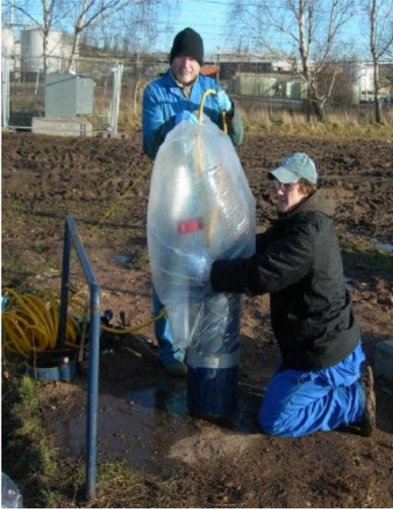
Figure 26. Attachment of the anaerobic gas bag.
