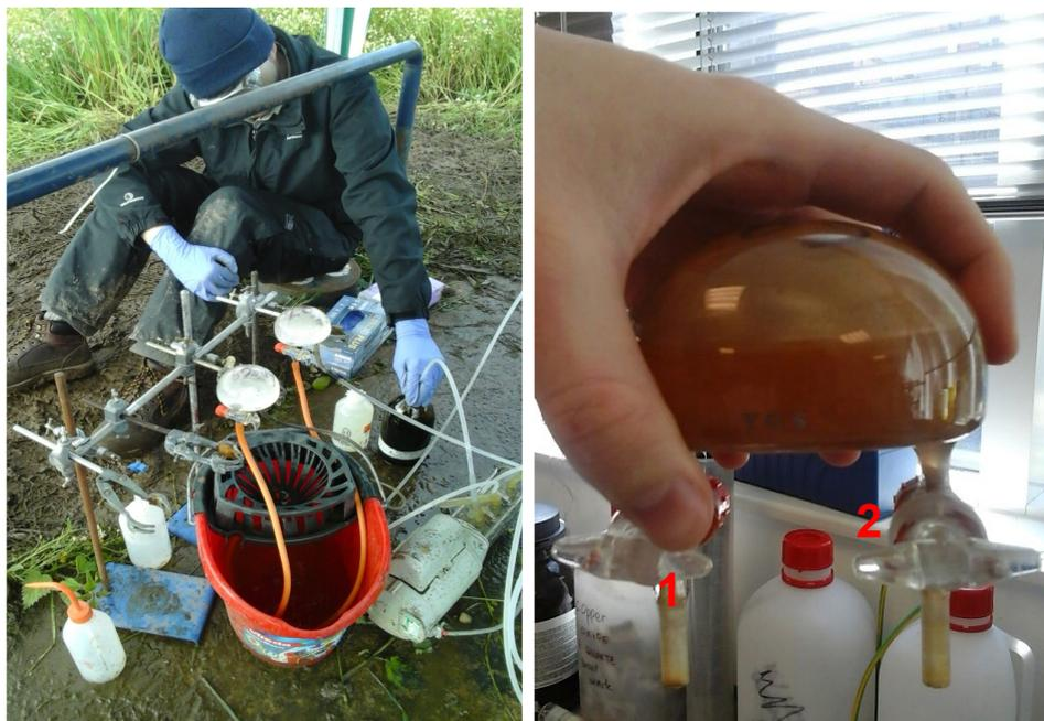
Figure 25. a) Blister trap set-up in the field and b) An inverted 'blister trap bubble' with (1) Inflow/outflow tubes (2) Valves. (Currently filled with a gas sample).
