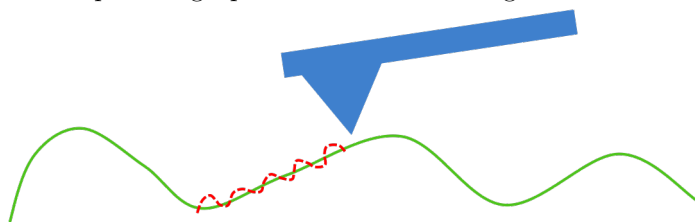
Figure 2.5: Diagram showing the AFM tip oscillating whilst in complete contact sample surface in force modulation mode.
