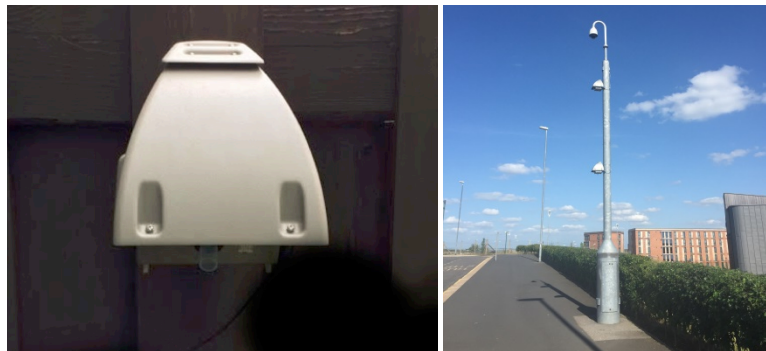
Figure 4- 8 The prototype of real-time wireless air-quality sensor (L) (City of York Council, 2016c), and the deployment on the lamppost on campus of the University of York in York (R)
