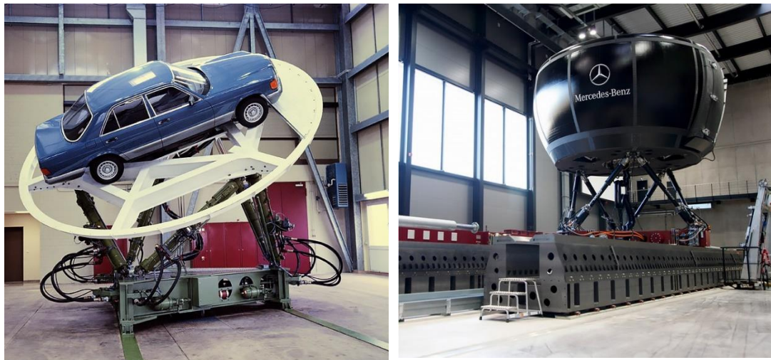
Figure 3-4. Daimler-Benz driving simulators 1985 (left) (Drosdol and Panik, 1985), 2010 (right) (Zeeb, 2010)
