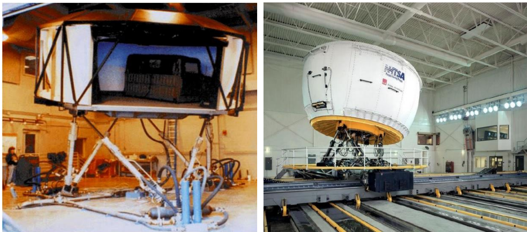
Figure 3-5. Iowa Driving Simulator 1992 (left) (Freeman et al., 1995) and, National Advanced Driving Simulator 2001 (right) (Clark, A. et al., 2001)
