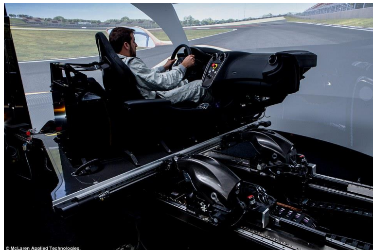
Figure 3-7. Vehicle Dynamics Simulator (VDS) of McLaren Applied Technologies (MTS), 2017
