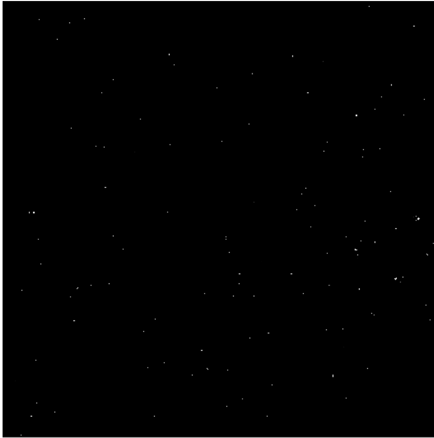
FIGURE 2.3. A single frame of holographic data projected gradient stack after a suitable threshold is applied. The bright point correspond to objects. This is used to locate locations of objects.
