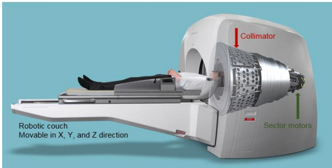
Figure 1.5: The GK Perfexion, that was introduced in 2006, had a fundamental change in design of the source housing and the collimator system. The tungsten collimator array is fixed and directly attached to the shielding block that houses the Co60 sources. Rather than being spherically arranged, the geometry of the Perfexion is conical. This allows linear movement of the sources between collimators.
