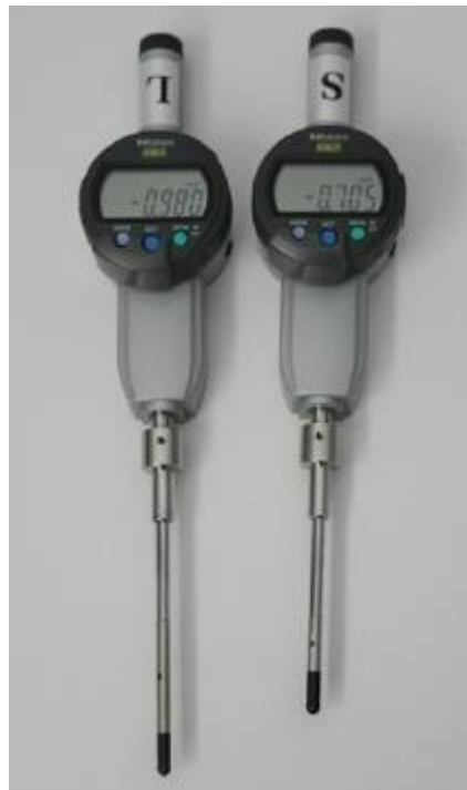
Figure 1.8: The gauge with the designed measurement start-position and a part which is slightly thicker than the measurement probe. This thicker part is used to guide the probe into the defined direction without swiveling. There is a long and a short probe since they have a limited measurement range. The indication is the difference to the calibrated zero position. The calibration takes place in the QA phantom (not imaged). (image from Sayer et al 2011, [95])
