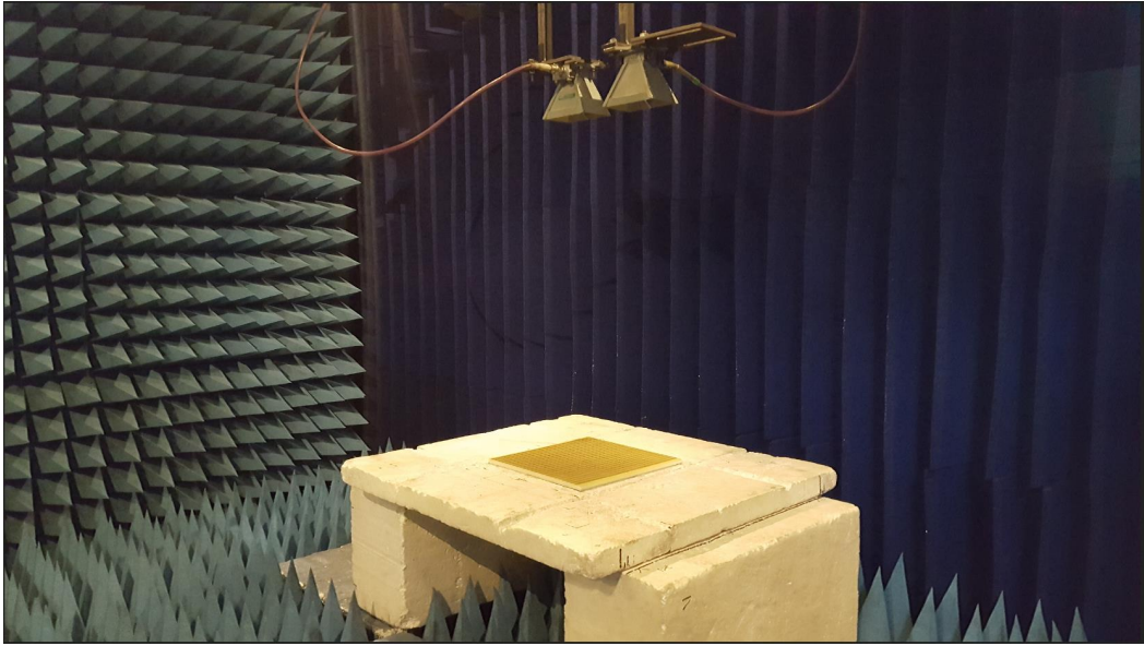
Fig. 6.5 Reflectivity measurement setup using NRL Arch.
