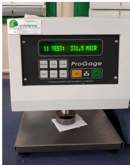
Figure 18: The ProGage thickness gauge used to measure the thickness of the samples.
