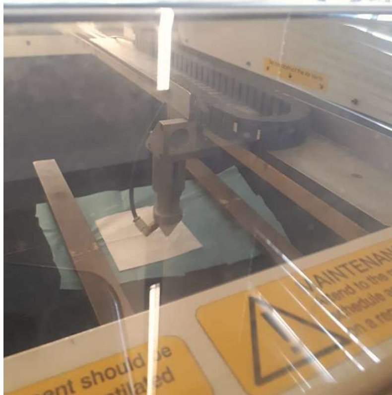
Figure 16: Demonstrates the laser cutter device in operation perforating pores into a scaffold which is held in place with weights.
