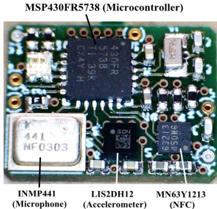
Fig. 5.2 The 12.5 mm × 10 mm × 1.5 mm printed circuit board
