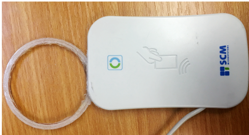
Fig. 4.1 The NFC reader with the extended ring-shaped antenna
