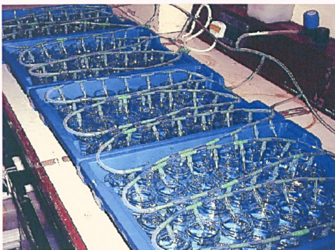
Figure 5.1. Photograph of experimental system used for quantifying leaf consumption by individuals of different shredder species.
