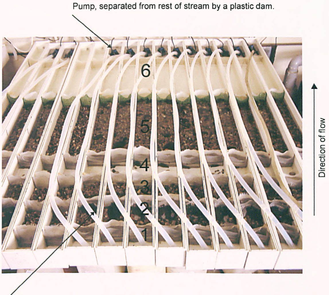
Plastic tubing for recirculating water
